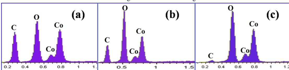
Figure S3 EDX elemental intensity of the NS arrays with different carbon content
