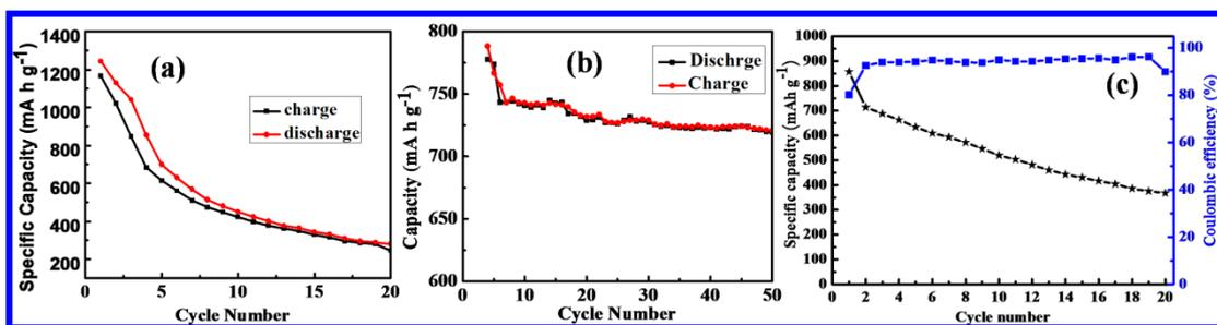
Figure. 5S (a): Figure. 5S (a): The capacity of the commercial  $\text{Co}_3\text{O}_4$  sample.(b): The capacity of  $\text{Co}_3\text{O}_4\text{-C}$  nanosheet array. (c) The capacity of  $\text{Co}_3\text{O}_4/\text{C}$  nanocomposites.
