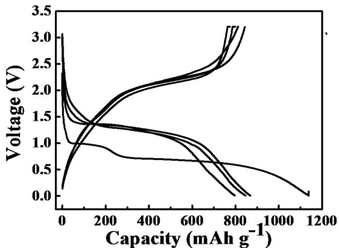
Figure. 4S the charge-discharge curves of  $\text{Co}_3\text{O}_4\text{-C}$  NS arrays for different cycles, the carbon content of the  $\text{Co}_3\text{O}_4\text{-C}$  NS is 16.5% and the mass of the electrode material is 2.94mg.
