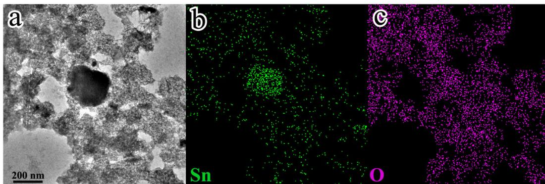
**Figure S5** TEM-EDS elemental mappings of bare SnO<sub>2</sub> nanocrystals in a de-lithiated state (3.0 V vs. Li<sup>+</sup>/Li) after 100 cycles: (a) TEM image, (b,c) EDS elemental mappings of Sn (green) and O (purple).
