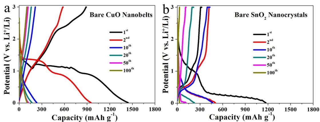
**Figure S3** The 1<sup>st</sup>, 2<sup>nd</sup>, 10<sup>th</sup>, 20<sup>th</sup>, 50<sup>th</sup>, and 100<sup>th</sup> discharge and charge curves for bare CuO nanobelts (a) and bare  $\text{SnO}_2$  nanocrystals.
