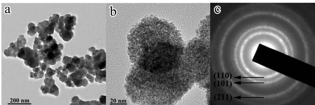
**Figure S2** TEM images and SAED pattern of bare SnO<sub>2</sub> nanocrystals.
