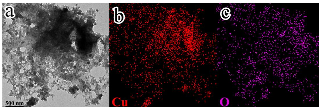
**Figure S4** TEM-EDS elemental mappings of bare CuO nanobelts in a de-lithiated state (3.0 V vs.  $\text{Li}^+/\text{Li}$ ) after 100 cycles: (a) TEM image, (b,c) EDS elemental mappings of Cu (red) and O (purple).
