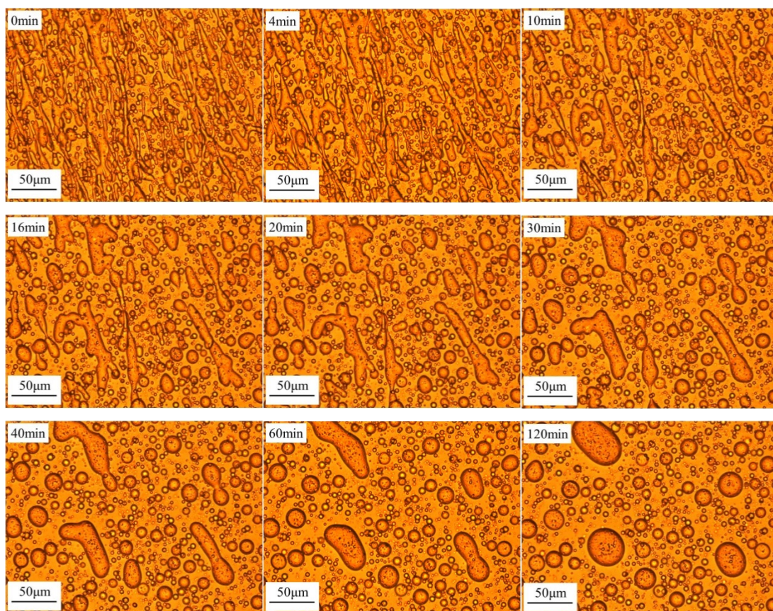
Figure 1 Morphology development of 2wt% A200 nano-silica particle (relative to the weight of PS phase) filled PP/PS 70/30 blend during annealing at 190°C
