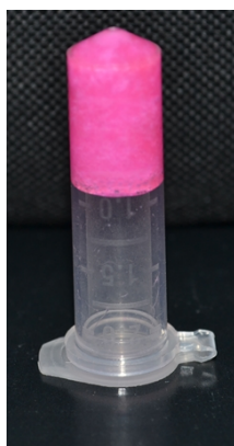
Fig 6. Self supporting hydrogel formation RATEA-F8 peptide in Tris. HCl buffer (pH =7.4). Rhodamine-B Dye was loaded inside the hydrogel which imparts the pink colour to the hydrogel.
