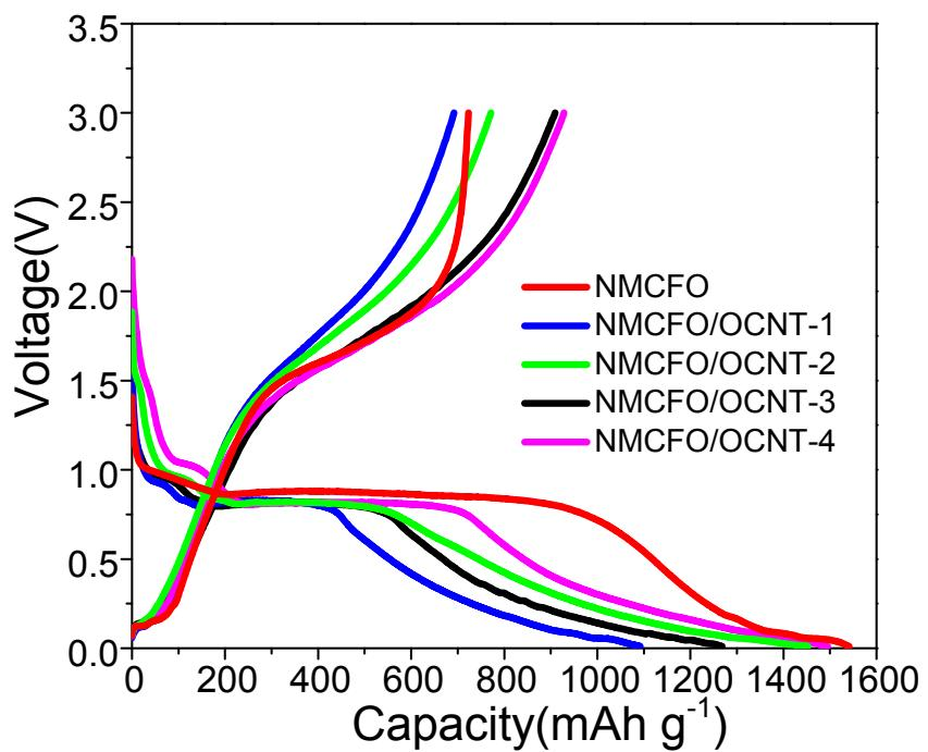
**Fig. S6** The first discharge-charge curves of NMCFO, NMCFO/OCNT-1, NMCFO/OCNT-2, NMCFO/OCNT-3, and NMCFO/OCNT-4.
