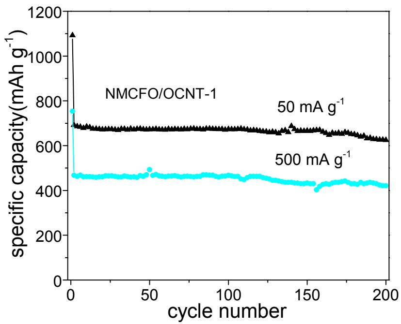
**Fig. S8** The cycling property of NMCFO/OCNT-1 at current densities of 50 and 500 mA g<sup>-1</sup>.
