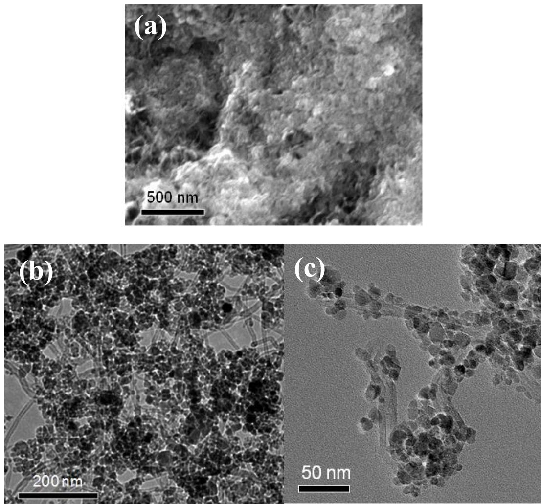
**Fig. S5** SEM image (a), and TEM images of NMCFO/OCNT-4 (b and c).
