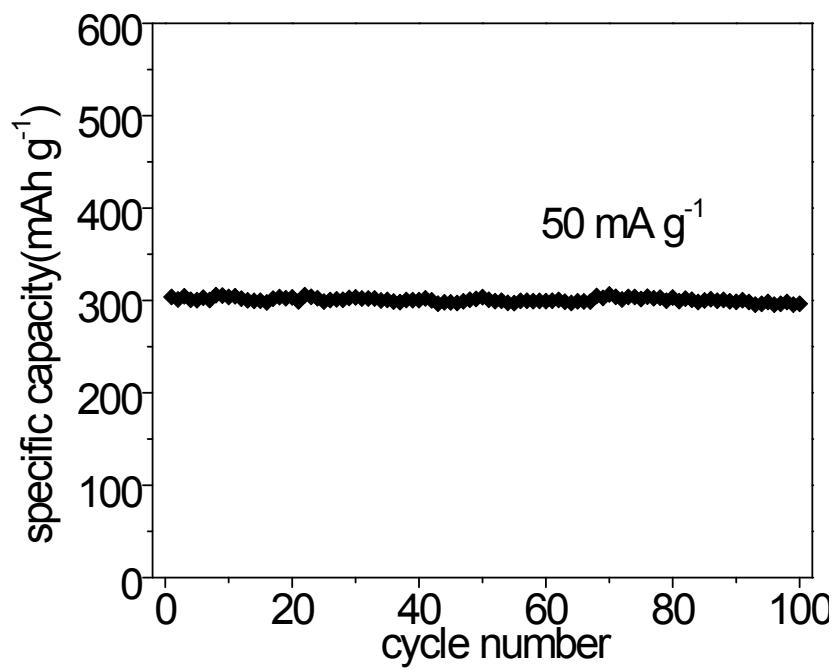
**Fig. S7** Cycling property of OCNT at a current density of  $50 \text{ mA g}^{-1}$ .
