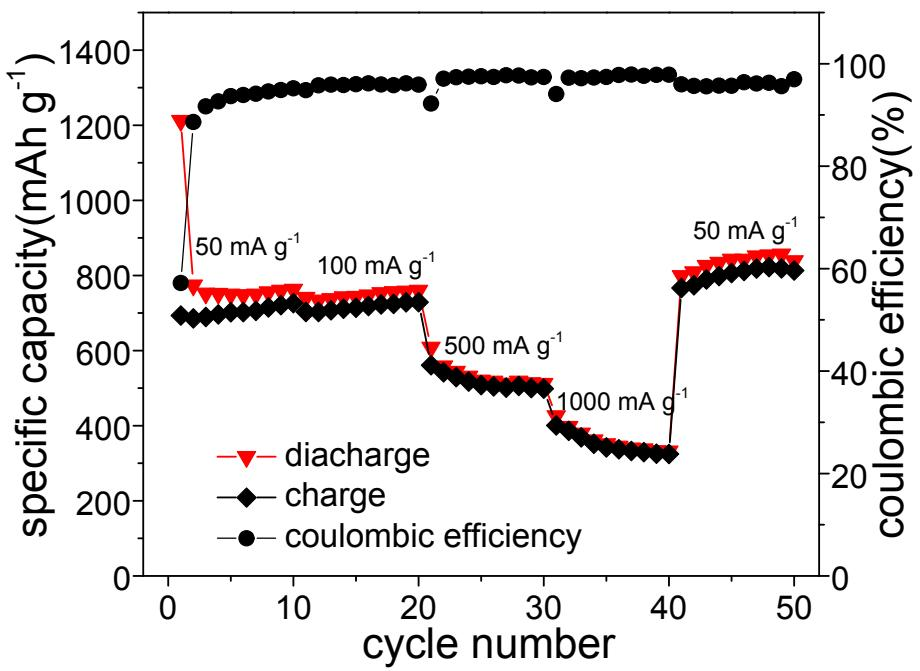
**Fig. S9** Rate performance of NMCFO/OCNT-2 at different current densities.
