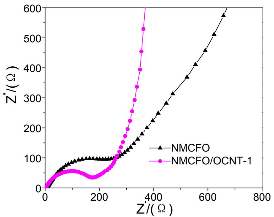
**Fig. S10** Nyquist plots of NMCFO and NMCFO/OCNT-1 samples at the electrode potentials from 0.70 to 0.10 V.
