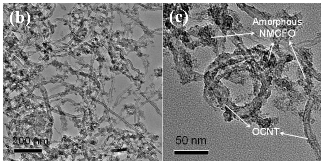
**Fig. S4** XRD pattern (a) and TEM images (b and c) of NMCFO/OCNT precursors.
