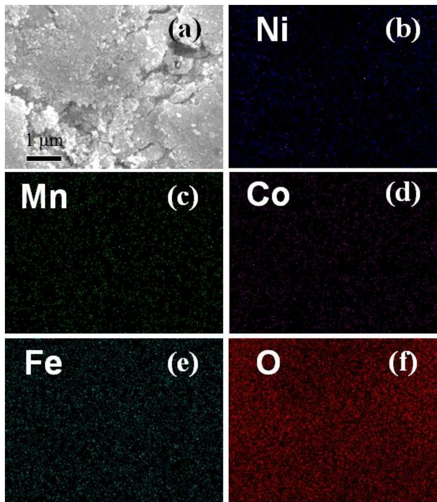
**Fig. S2** Elemental mapping images of Ni, Mn, Co, Fe, and O for NMCFO nanoparticles.
