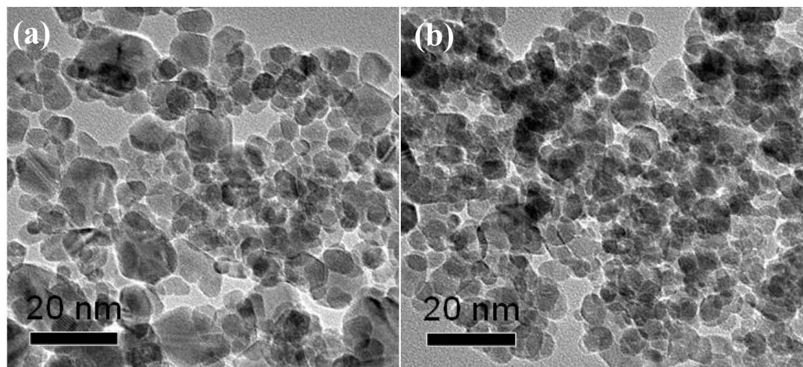
**Fig. S3** TEM images of (a)  $\text{Ni}_{0.2}\text{Mn}_{0.4}\text{Co}_{0.4}\text{Fe}_2\text{O}_4$  and (b)  $\text{Ni}_{0.4}\text{Mn}_{0.4}\text{Co}_{0.2}\text{Fe}_2\text{O}_4$ .
