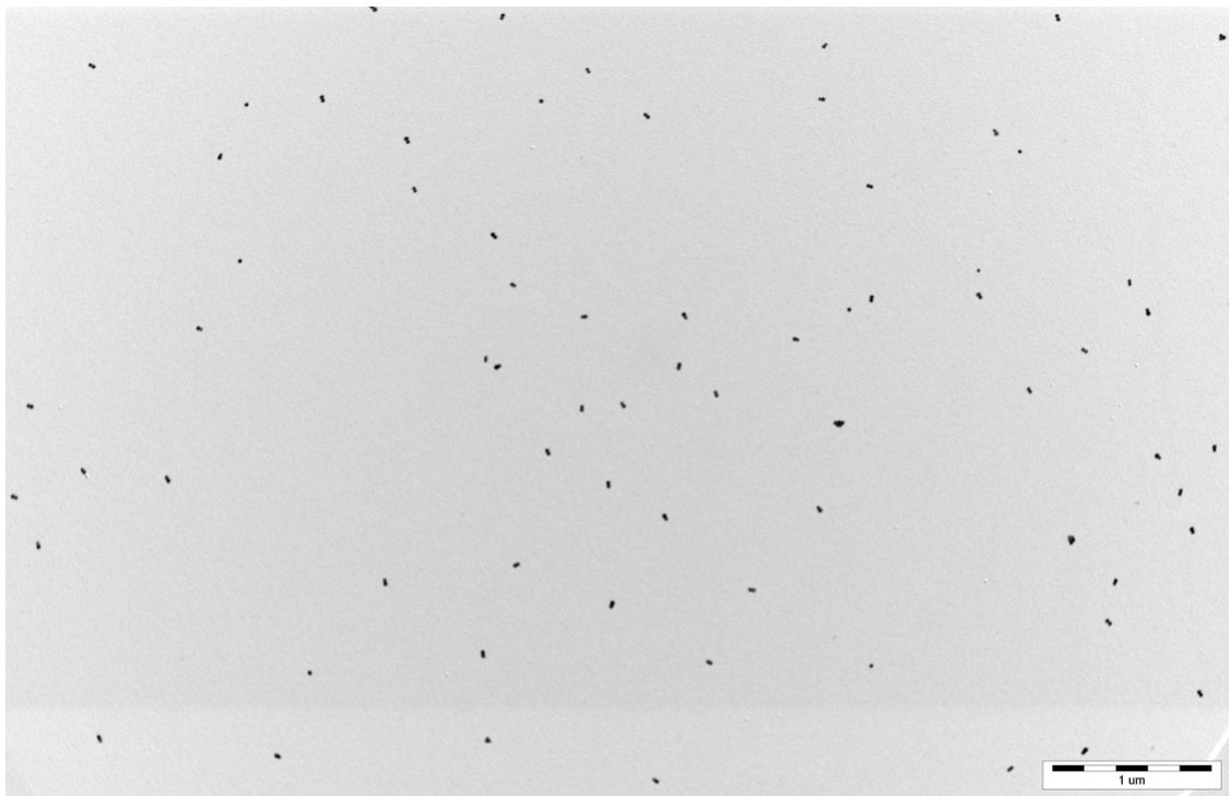
Fig. S4 TEM of the two-AuNPs NAs prepared by the dsDNA self-assembly strategy.
