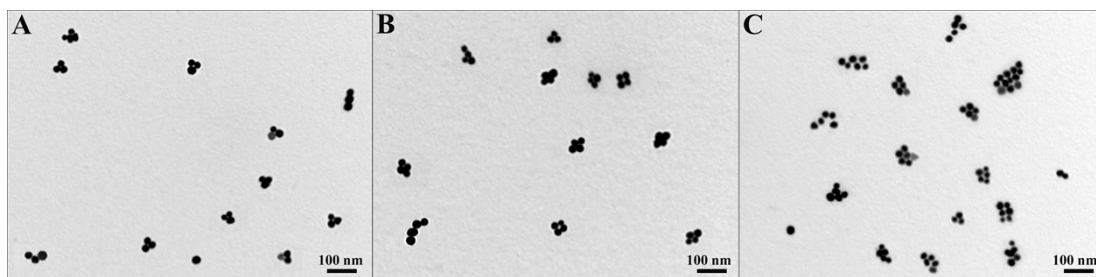
Fig. S5 Large scale TEM images of the Au NAs with (A) three, (B) four and (C) five Au NPs.
