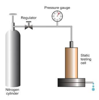
**Figure S1:** Liquid entry pressure test setup.
