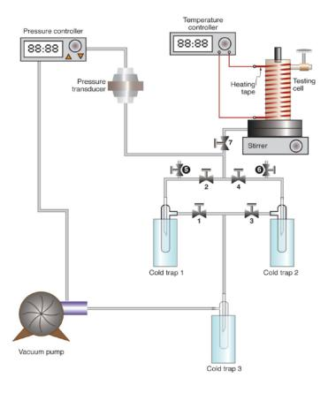
Figure S2: Vacuum membrane distillation experimental setup.
