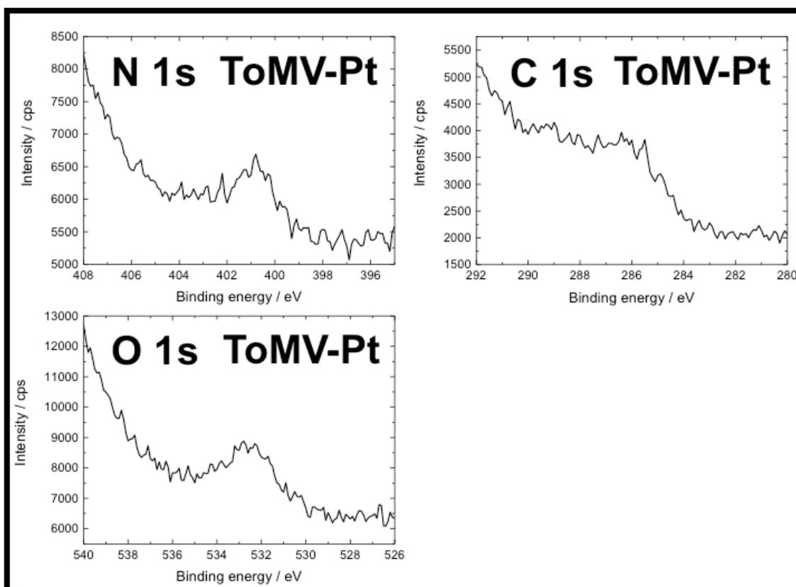
**Figure S12** : N 1s (~401 eV), C 1s (~285 eV) and O 1s (~532 eV) XPS spectra of Pt-NT.
