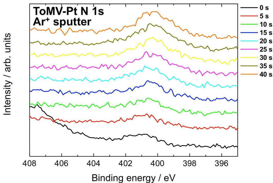
**Figure S14:** N1s XPS spectra of Pt-NT over 40 s of sputtering with readings taken at 5 s intervals. Increases in the peak area and intensity at ~401 eV were observed over time, indicating that nitrogenous impurities can be removed by Ar<sup>+</sup> sputtering treatment.
