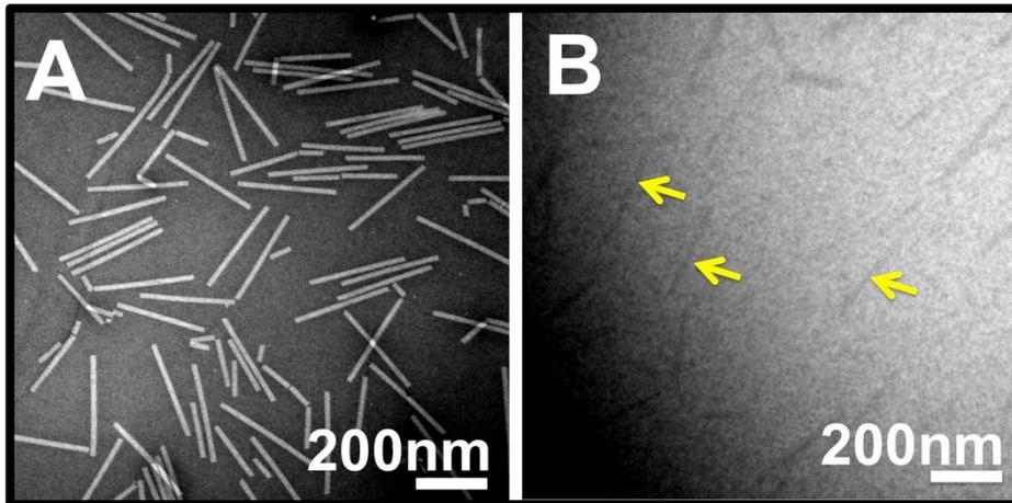
**Figure S3.** Comparison of Pt NTs before and after heating. TEM images were acquired from identical areas of the SiN membrane before and after annealing of ToMV-Pt at 400 °C in air for 4 h. Images A, B and C are before heating, showing outer diameter of 50(±5) nm. A', B', and C' show the same areas after heating.
