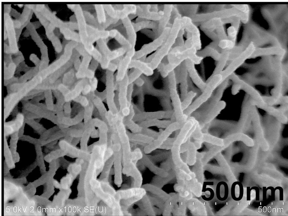
**Figure S5.** FE-SEM image shows Pt-NT synthesis at 400 °C in air overnight; no visible damage was observed.
