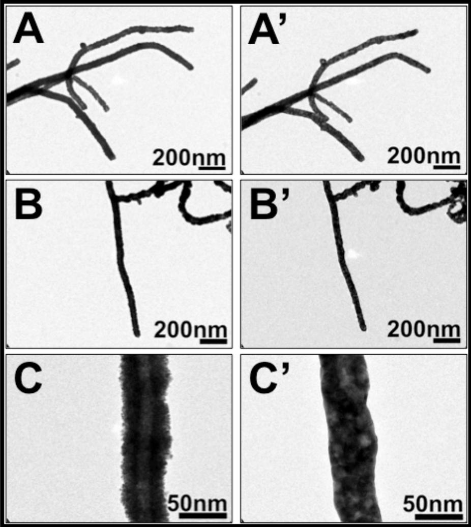
**Figure S4.** FE-SEM image shows that Pt-NTs have retained their morphology even after sudden cooling. Freshly prepared purified ToMV-Pt was loaded onto a silicon oxide wafer and annealed at 300 °C in air for 4 h, and cooled in atmospheric air to 25 °C over ~5 min. No visible damage is observed .
