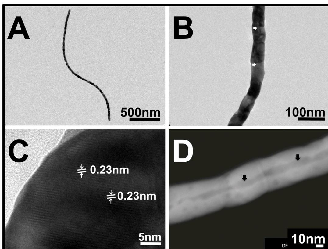
**Figure S7.** 2D-STEM dark field image showing Pt-NTs produced after annealing of ToMV-Pt. The hollow central channel (black line) and cavities throughout (black patches) are visible.
