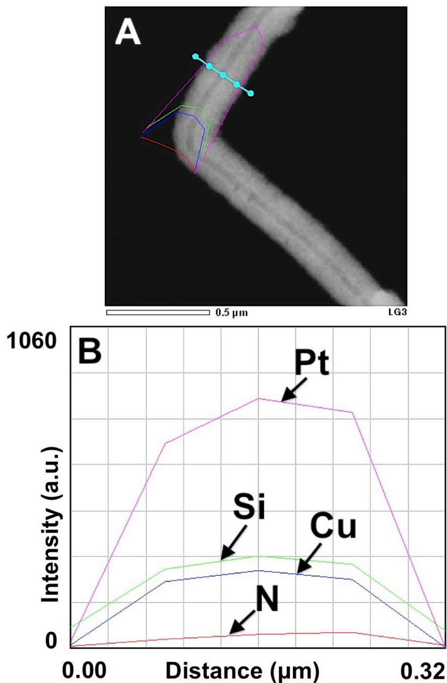
**Figure S9.** EDS line scanning of Pt-NT in STEM dark field mode; (A) Profiles were taken along the cyan colored line with five spots chosen for analysis. (B) The profile line (pink) for the middle three spots showed high platinum intensities. Silicon (Si) and nitrogen (N) signal arises from SiN membrane and carbon (C) and oxygen (O) signals mainly from TEM chamber respectively. A barium TEM holder is used to minimize the copper noise.
