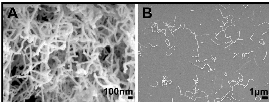
**Figure S2.** TEM image of ToMV stained with 3 % PTA on a SiN before (A) and after (B) heating at 250 °C in air for 30 mins. Arrows show a “shadow” left behind after decomposition of the ToMV.
