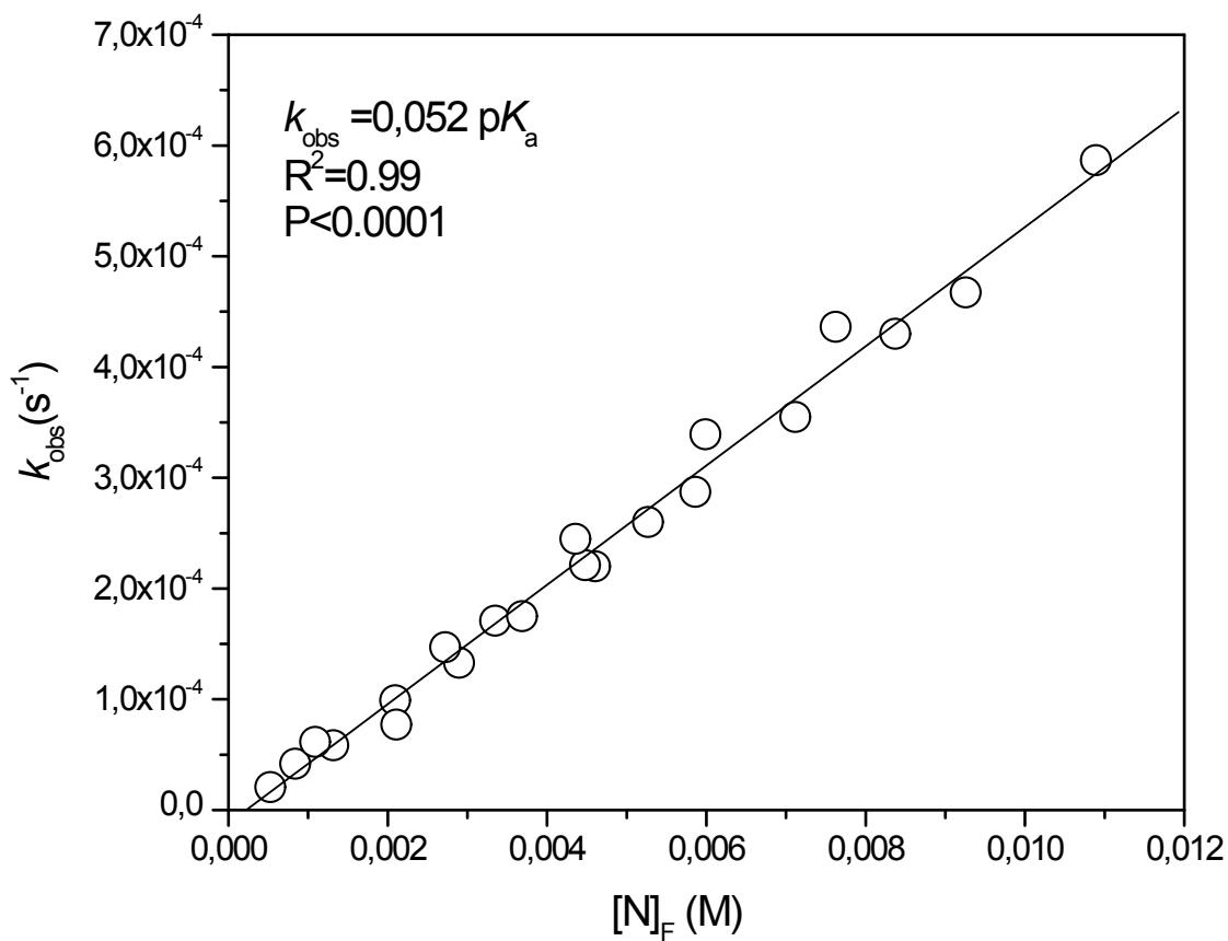
**Figure S3.**  $k_{\text{obs}}$  vs. free concentration of 4-chlorobenzoic hydrazide in water, at 25.0 °C, ionic strength 0.2 M (KCl).
