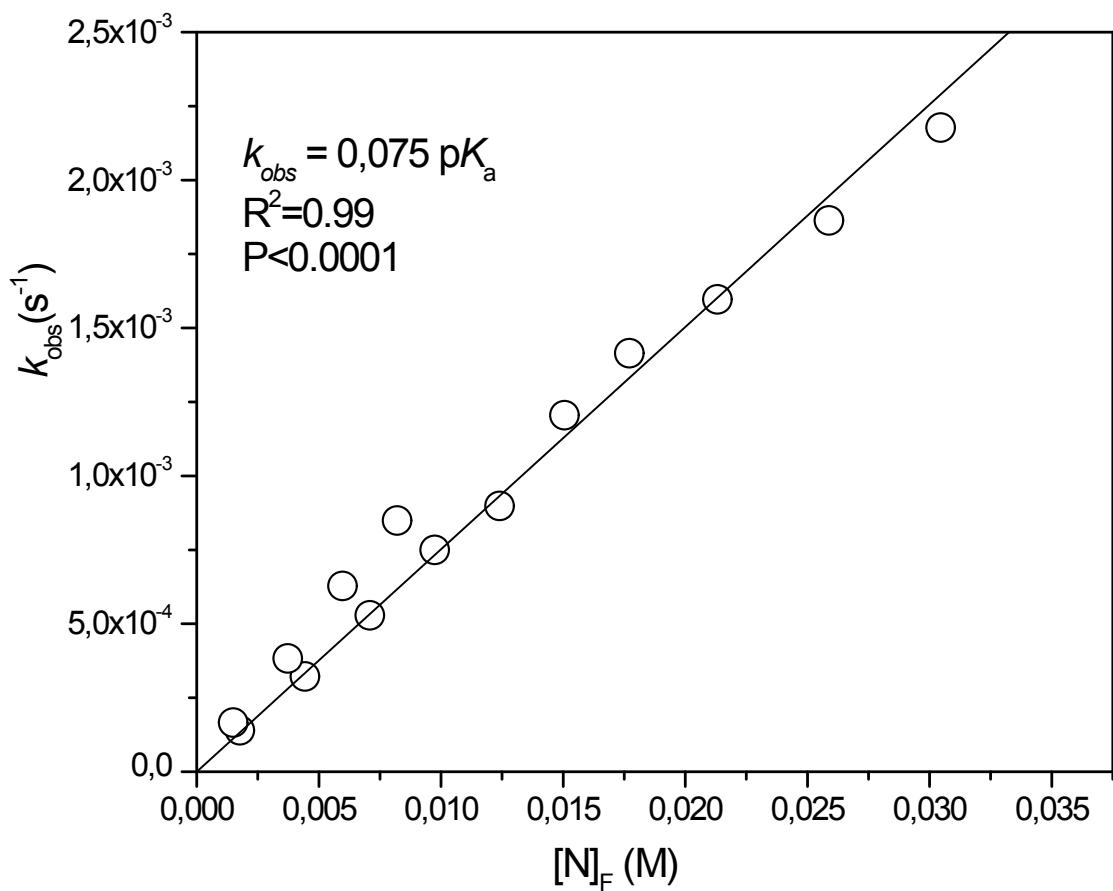
**Figure S1.**  $k_{obs}$  vs. free concentration of benzoic hydrazide in water, at 25.0 °C, ionic strength 0.2 M (KCl).
