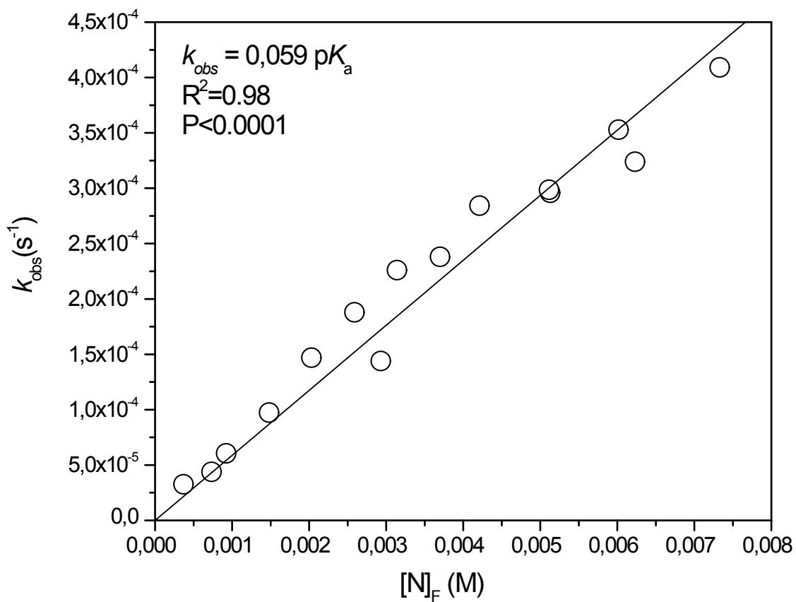
**Figure S5.**  $k_{\text{obs}}$  vs. free concentration of 4-(trifluoromethyl)benzhydrazide in water, at 25.0 °C, ionic strength 0.2 M (KCl).
