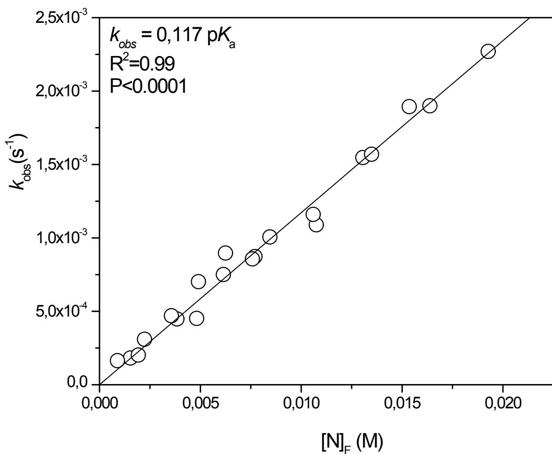
**Figure S2.**  $k_{obs}$  vs. free concentration of *p*-toluic hydrazide in water, at 25.0 °C, ionic strength 0.2 M (KCl).
