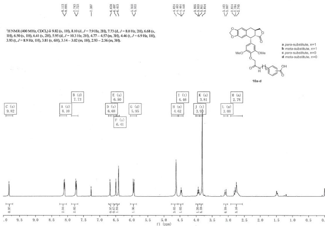
**Figure S9.**  $^1\text{H}$  NMR Spectrum of **10d** (400 MHz,  $\text{CDCl}_3$ )
