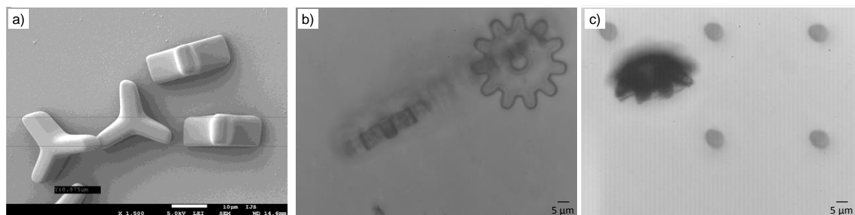
ESI_1. (a) SEM image of SU-8 microstructures \sim 9\ \mu\text{m} high, (b) bright field image of SU-8 microstructures \sim 9\ \mu\text{m} thick, (c) bright field image of magneto-responsive microgears \sim 9\ \mu\text{m} thick.
