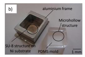
**ESI\_2**. a) The fabrication step where the aluminium frame is used. b) SU-8 master template on a nickel substrate with the aluminium frame on it (left); it was used to produce a cuboidal PDMS mold with the microhollow structure in the center (right).
