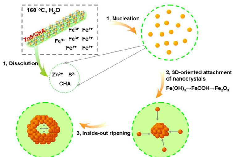
**Scheme S1.** Scheme for synthesis of the hollow single-crystalline  $\alpha$ -Fe<sub>2</sub>O<sub>3</sub> nanospheres.
