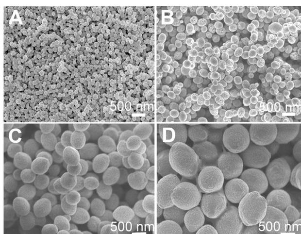
**Fig. S6** SEM images of the different size  $\text{Fe}_2\text{O}_3$  nanospheres with multiplied  $\text{Fe}^{3+}$  source (A) 0.16 g; (B) 0.32 g; (C) 0.48 g and (D) 0.64 g  $\text{FeCl}_3 \cdot 6\text{H}_2\text{O}$ .
