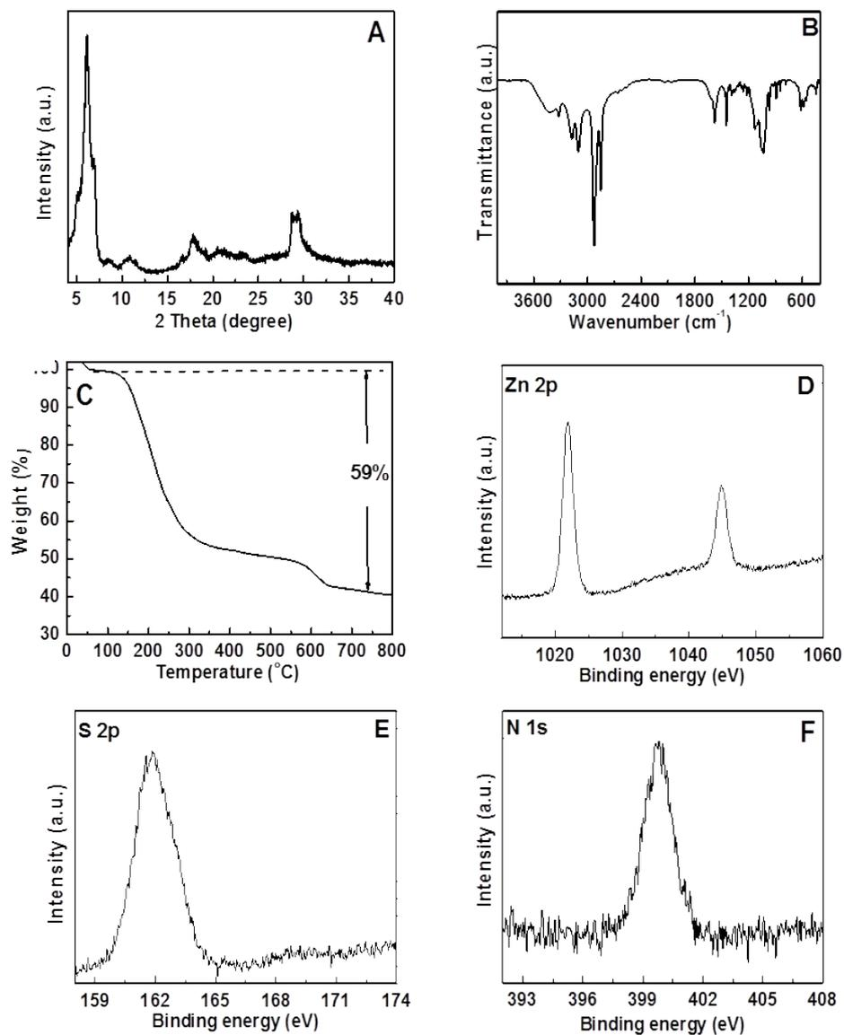
**Fig. S1** (A) XRD pattern; (B) IR spectrum; (C) TG analysis; high resolution XPS spectra of (D) Zn 2p, (E) S 2p and (F) N 1s for the ZnS-CHA nanocomposite.
