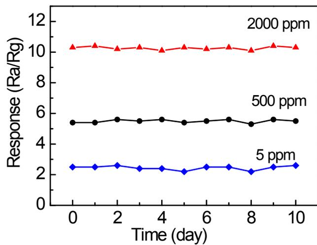
**Fig. S10** Stability sensing measurement to ethanol of the single-crystalline hollow  $\text{Fe}_2\text{O}_3$  nanospheres.
