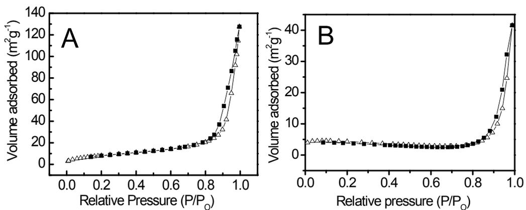
**Fig. S8** Nitrogen adsorption-desorption isotherm of (A) the single-crystalline hollow  $\text{Fe}_2\text{O}_3$  nanospheres and (B)  $\text{Fe}_2\text{O}_3$ -1.
