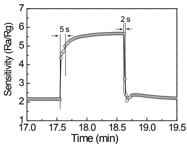
**Fig. S9** Magnification curve of the single-crystalline hollow  $\text{Fe}_2\text{O}_3$  nanospheres towards 500 ppm ethanol.
