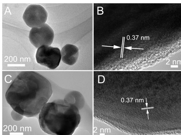
**Fig. S7** (A) TEM and (B) HRTEM images of the  $\text{Fe}_2\text{O}_3$  obtained at 6 h; (C) TEM and (D) HRTEM images of the  $\text{Fe}_2\text{O}_3$ -1 (In control experiment section (1)).
