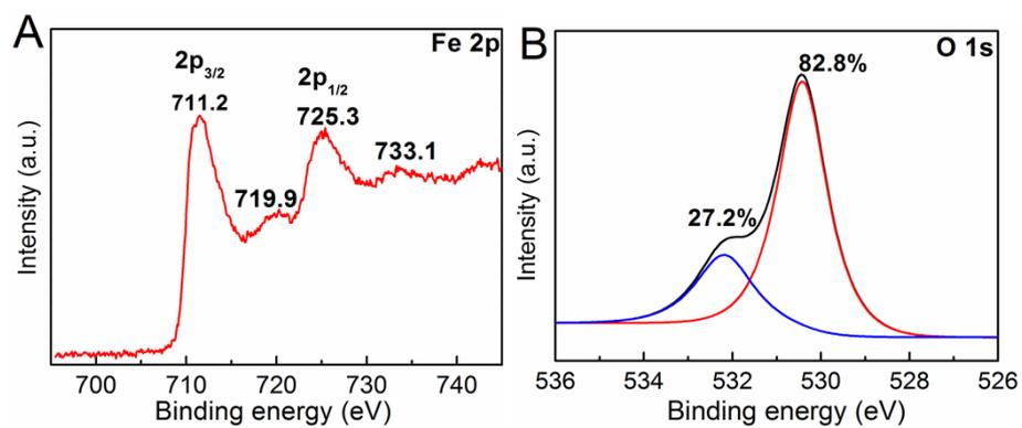
**Fig. S4** High resolution XPS spectra (A) Fe 2p and (B) O 1s of the single-crystalline hollow  $\text{Fe}_2\text{O}_3$ .
