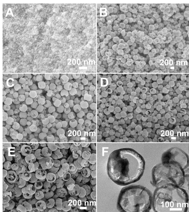
**Fig. S3** SEM images of the products obtained at (A) 30 min, (B) 1 h, (C) 6 h, (D) 8 h (E) 24 h, and (F) low magnification TEM for 24 h.
