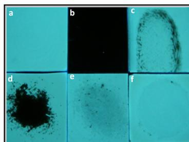
**Fig. S4** Photographs of TCEPA-coated test strips under different experimental conditions. (a)blank. (b) After dipping into solutions of PA in THF ( $1 \times 10^{-3}$  M). (c) Thumb impression after rubbing with PA crystals. (d) PA
