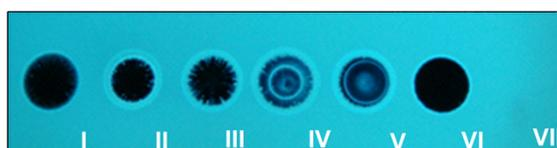
**Fig. S6** Photograph of the fluorescence quenching of TCEPA-coated test strips by PA on contact mode (10  $\mu\text{L}$  of PA with a spot area of  $\sim 0.2 \text{ cm}^2$ ) when viewed under 365 nm UV illumination., (I)  $1 \times 10^{-3} \text{ M}$ , (II)  $1 \times 10^{-5} \text{ M}$ , (III)  $2 \times 10^{-7} \text{ M}$ , (IV)  $1 \times 10^{-9} \text{ M}$ , (V)  $1 \times 10^{-11} \text{ M}$ , (VI)  $1 \times 10^{-13} \text{ M}$ , (VII) blank.
