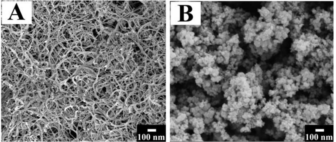
Figure S1. SEM images of (A) MWCNT, (B) MnO<sub>2</sub>, deposited by EPD.
