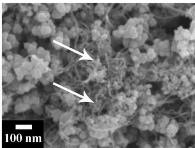
Figure S5. SEM image of MnO<sub>2</sub>-MWCNT composite, prepared without dispersants. Arrows show MWCNT agglomerate.
