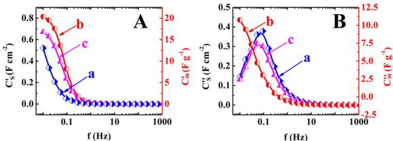
Figure S8. Frequency dependences of components of complex capacitance, calculated from the impedance data (A)  $C'$  and (B)  $C''$  for (a) pure AC without CB, and composites, containing (b) 90% AC and 10% CB (c) 85% AC and 15% CB.
