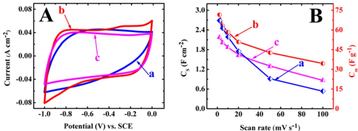
Figure S6. (A) Cyclic voltammograms at a scan rate of  $20 \text{ mV s}^{-1}$  and (B) specific capacitances versus scan rate for (a) pure AC without CB, and composite electrodes, containing (b) 90% AC and 10% CB (c) 85% AC and 15% CB in  $0.5\text{M}$  aqueous  $\text{Na}_2\text{SO}_4$  electrolyte.
