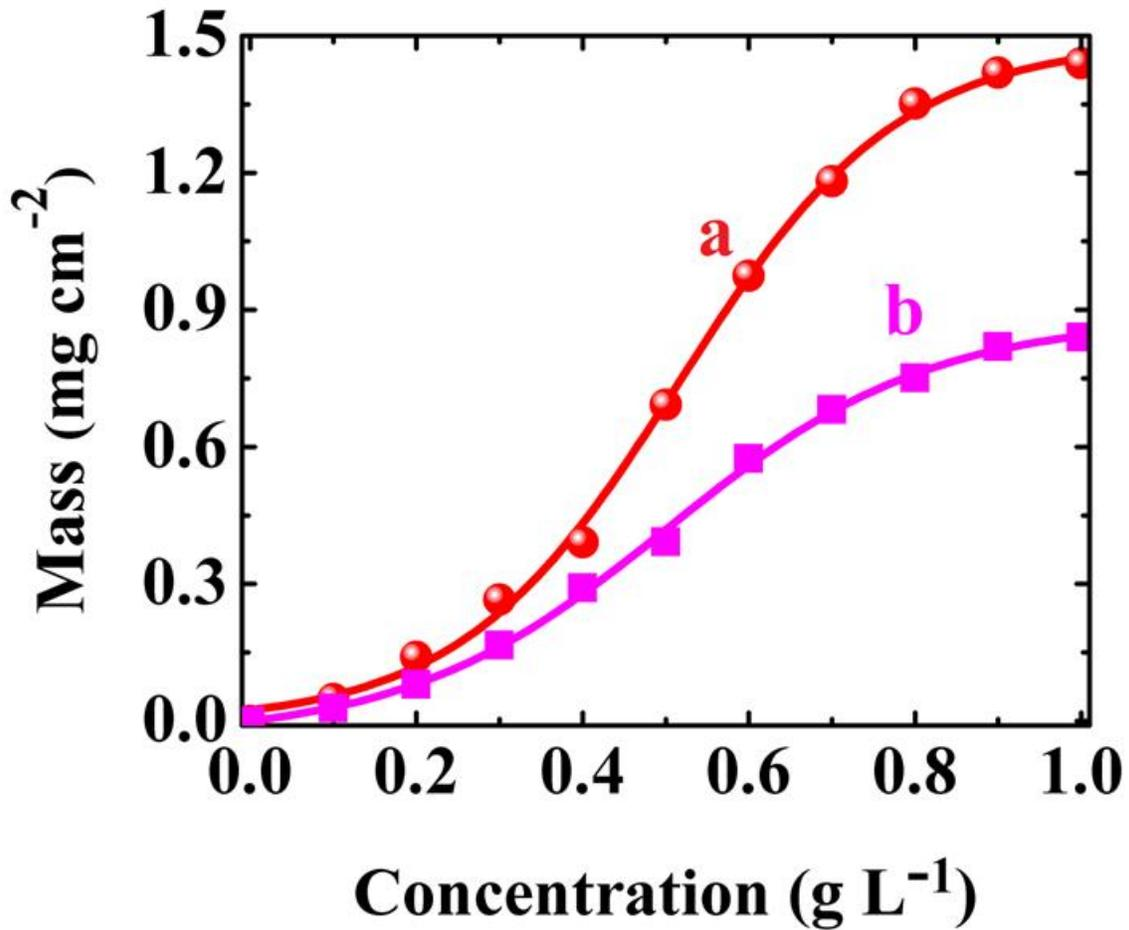
Figure S3. Comparison of the deposition yield obtained from 1 g L<sup>-1</sup> MWCNT suspension in water at a deposition voltage of 20 V and deposition time of 3 min: (a) versus BAC concentration and (b) versus CTAB concentration.
