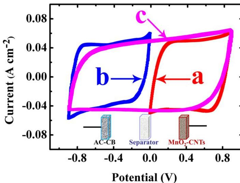
Figure S9. Cyclic voltammograms of (a)  $\text{MnO}_2$ -MWCNTs composite electrode, (b) AC-CB composite electrode and (c) the cell composed by the two electrodes above at scan rate of  $20 \text{ mV s}^{-1}$  in  $0.5\text{M}$  aqueous  $\text{Na}_2\text{SO}_4$  electrolyte. The inset shows configuration of the device.
