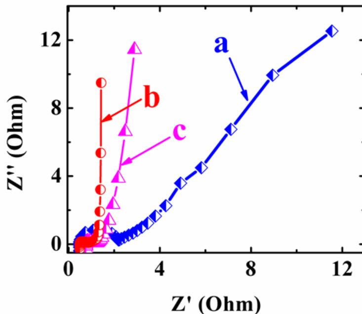
Figure S7. Nyquist plot of complex impedance for (a) pure PICA without CB and composite electrodes, containing (b) 90% AC and 10% CB (c) 85% AC and 15% CB in  $0.5\text{M}$  aqueous  $\text{Na}_2\text{SO}_4$  electrolyte.
