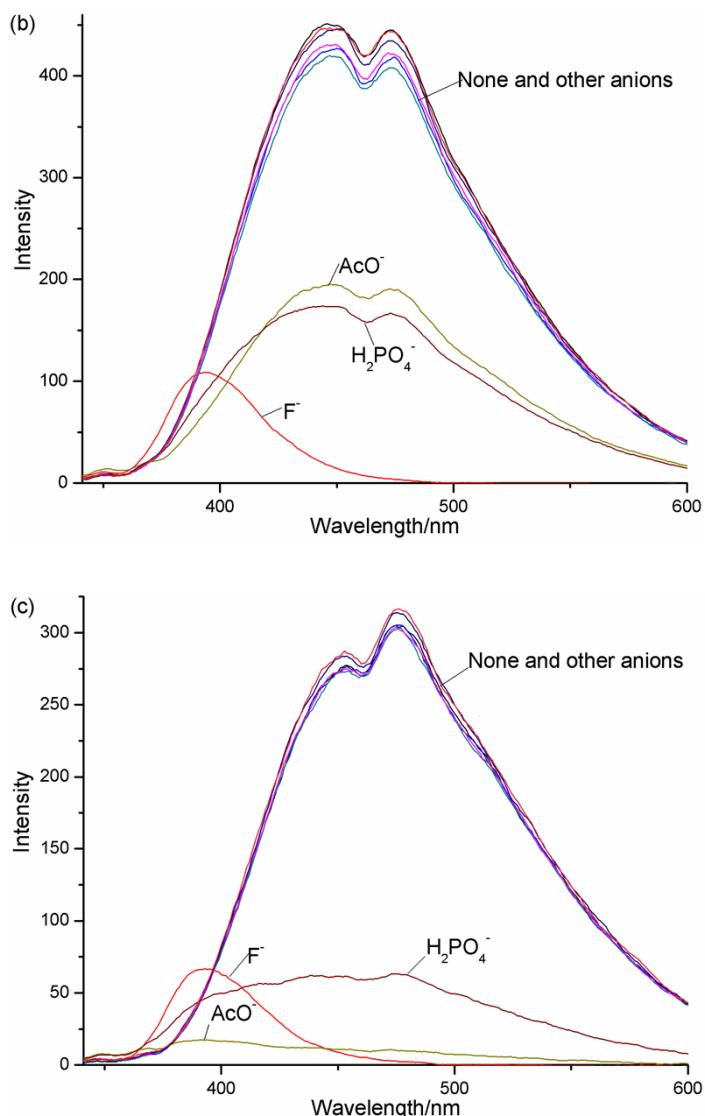
**Fig. S3.** Fluorescence responses of **3-5** (10  $\mu\text{M}$ ) to various anions (50  $\mu\text{M}$ ) in  $\text{CH}_3\text{CN}$ .  $\lambda_{\text{ex}}=331\text{nm}$ . (a) compound **3**, (b) compound **4**, (c) compound **5**.
