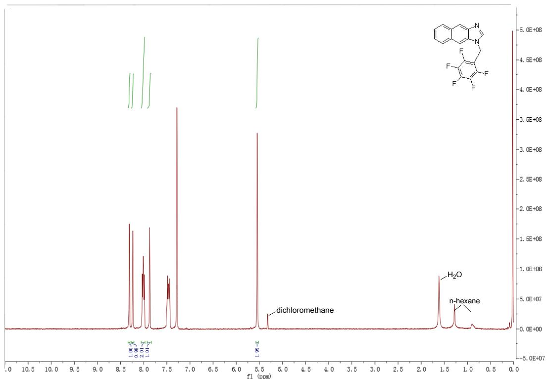
**Fig. S11.**  $^1\text{H}$ -NMR of compound **12** in  $\text{CDCl}_3$ .
