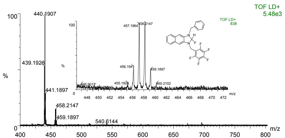
**Fig. S6.** MALDI-TOF (LD+) spectrum of compound 4 with 5 equiv. F<sup>-</sup> addition.
