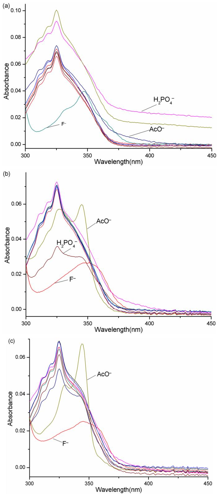
**Fig. S1.** Absorbance spectra of compound **3-5** (10  $\mu\text{M}$ ) in acetonitrile with different anions (50  $\mu\text{M}$ ,  $\text{Cl}^-$ ,  $\text{Br}^-$ ,  $\text{I}^-$ ,  $\text{AcO}^-$ ,  $\text{H}_2\text{PO}_4^-$ , and  $\text{HSO}_4^-$ , as  $n\text{-Bu}_4\text{N}^+$  salts). (a) compound **3**, (b) compound **4**, (c) compound **5**.
