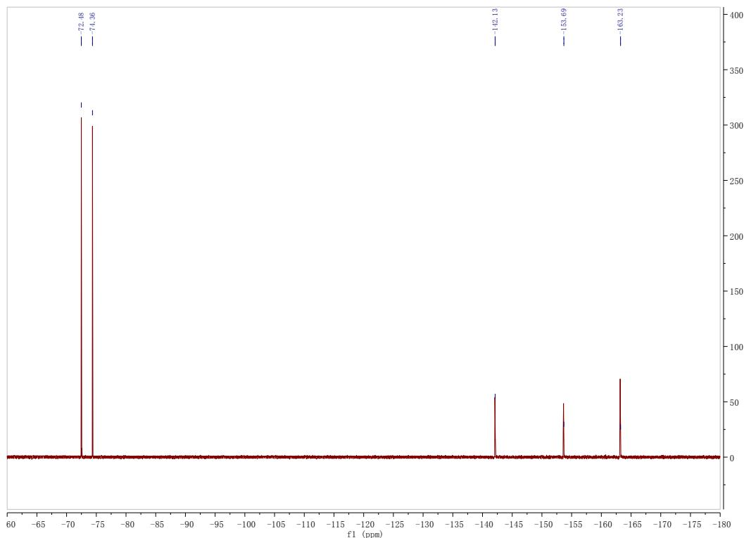
**Fig. S22**  $^{19}\text{F}$ -NMR of compound **5** in  $\text{CD}_3\text{CN}$ .
