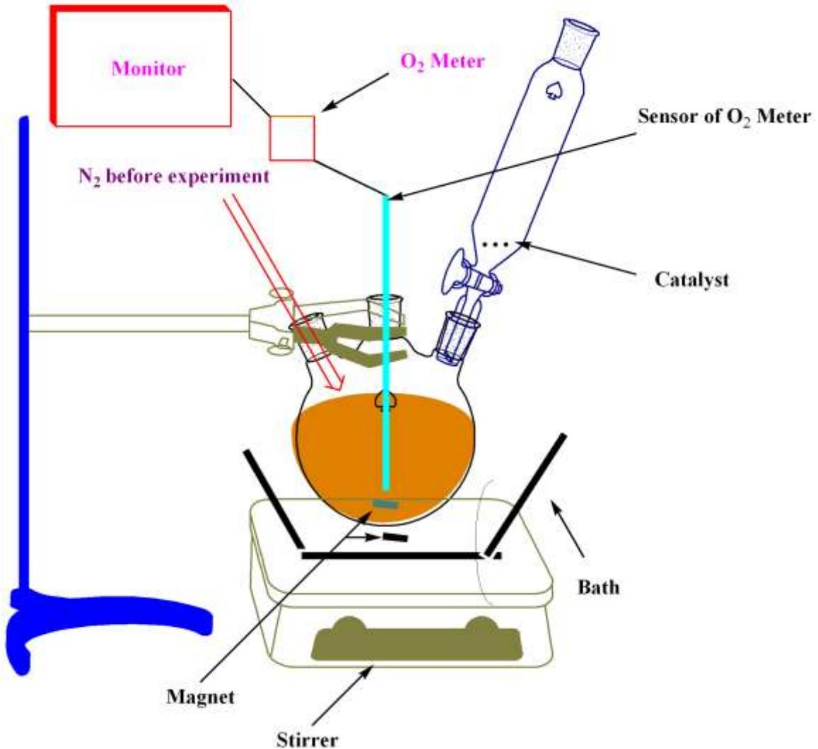
Scheme S1 Set up for water-oxidation experiments.
