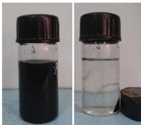
Figure. 5 a. Cu-Ni bimetallic catalyst suspended in ethyl acetate after reaction completion; 5 b. Cu-Ni bimetallic catalyst was collected by magnetic bar.
