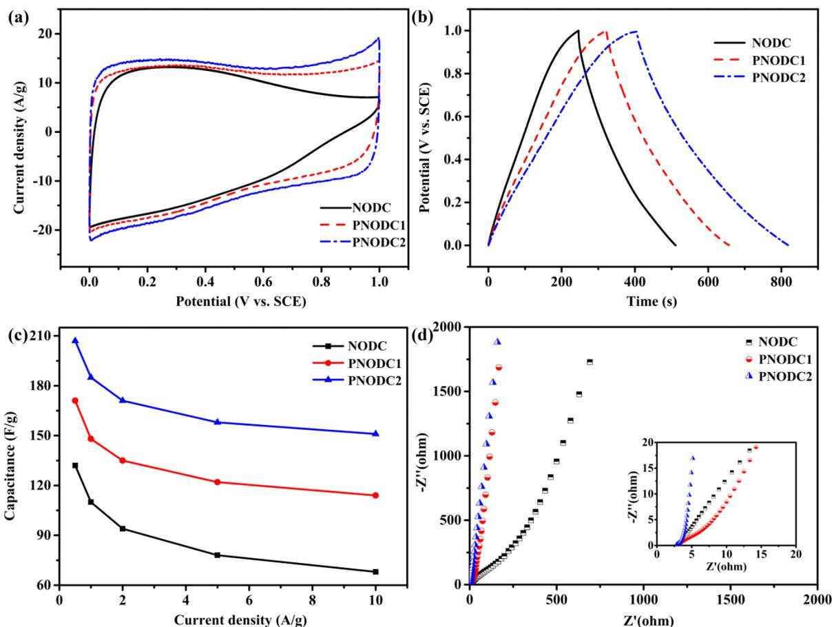
Figure S4. (a) CV curves at 100 mV/s; (b) galvanostatic charge and discharge curves; (c) specific capacitance vs. current density plots from 0.5 A/g to 10 A/g; (d) Nyquist plots, the inset is the magnified view of the high-frequency zone, of all carbon samples in three electrode system in the 1 M  $\text{H}_2\text{SO}_4$  solution.
