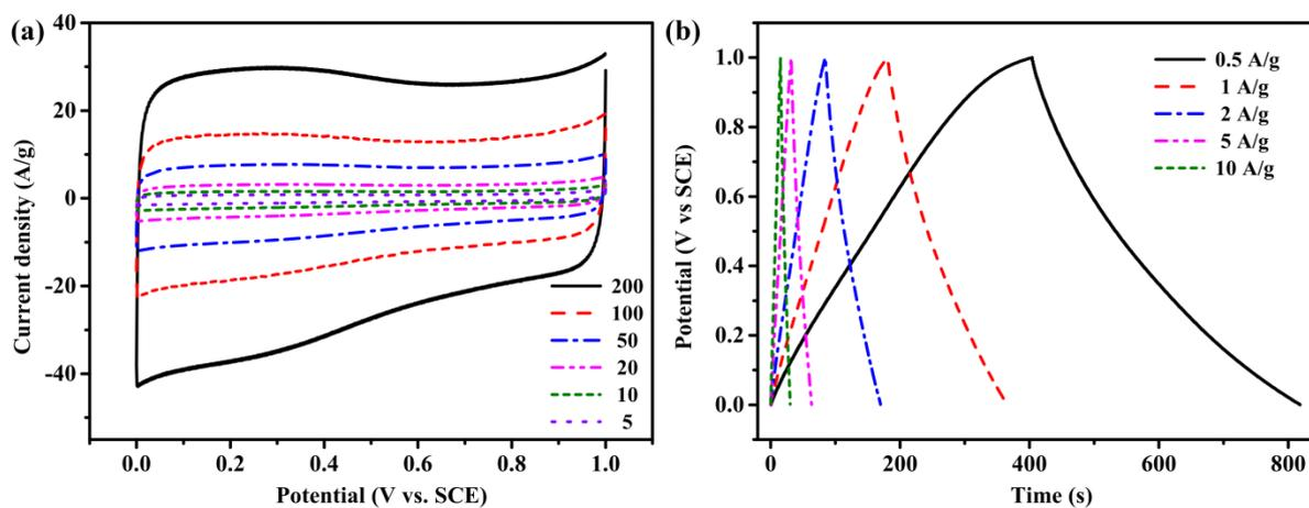
Figure S5. (a) CV from 5 mV/s to 200 mV/s and (b) galvanostatic charge and discharge curve of PNODC2 in three electrode system in 1 M  $\text{H}_2\text{SO}_4$  electrolyte.
