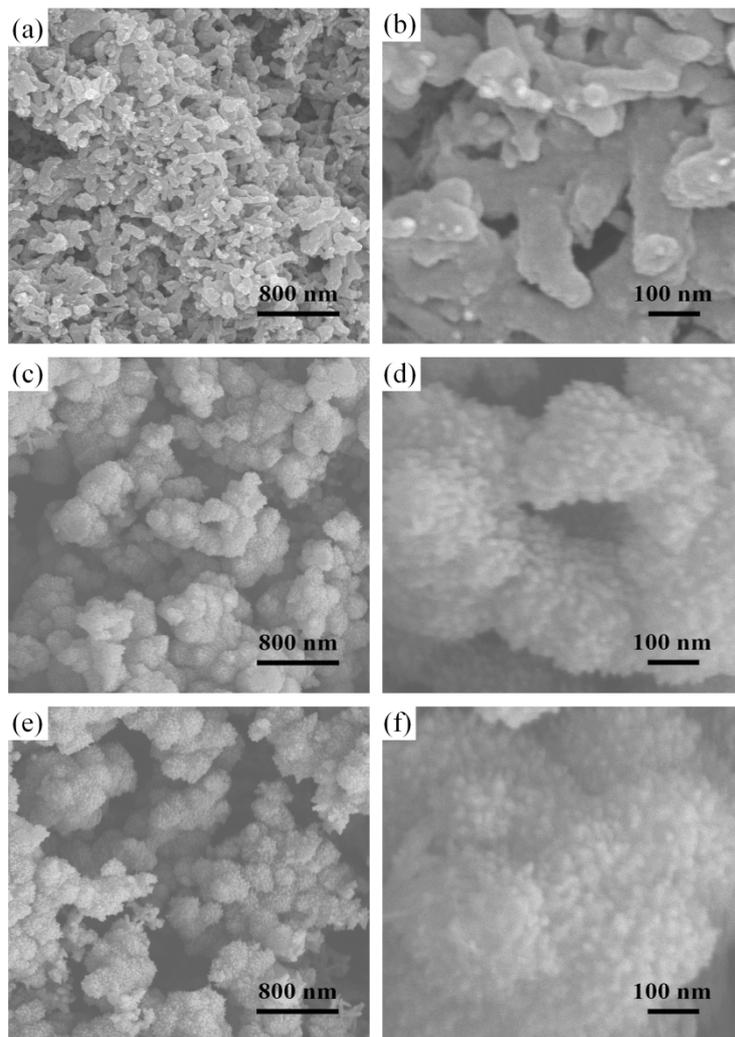
Figure S2. SEM images of (a-b) HCl-PANI, (c-d) PA-PANI1 and (e-f) PA-PANI2.
