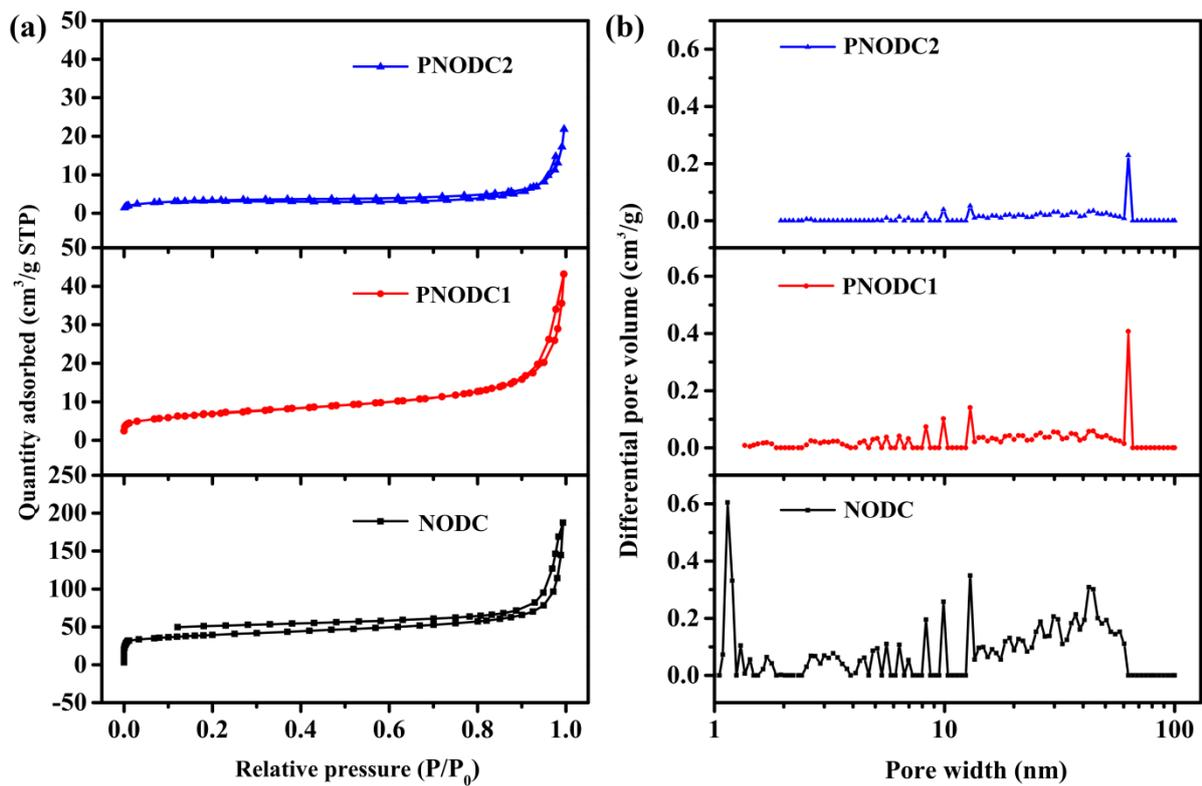
Figure S3.  $\text{N}_2$  sorption isotherms and PSD by NLDFIT of NODC, PNODC1 and PNODC2.
