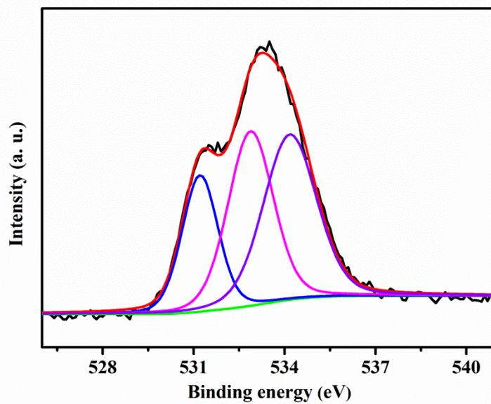
Figure S6. O spectrum of carbon materials after cycling at 10 A/g for 10000 cycles.
