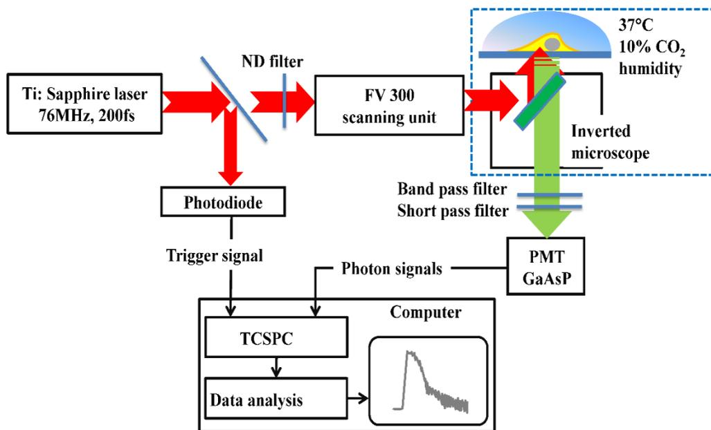
**Supplementary Fig. 2** Schematic view of FLIM setup. The Inverted microscope was installed inside an incubation chamber (fitted with 10% CO<sub>2</sub>, 37°C and approximate 90% humidity controller) for live cell imaging under physiological conditions,.
