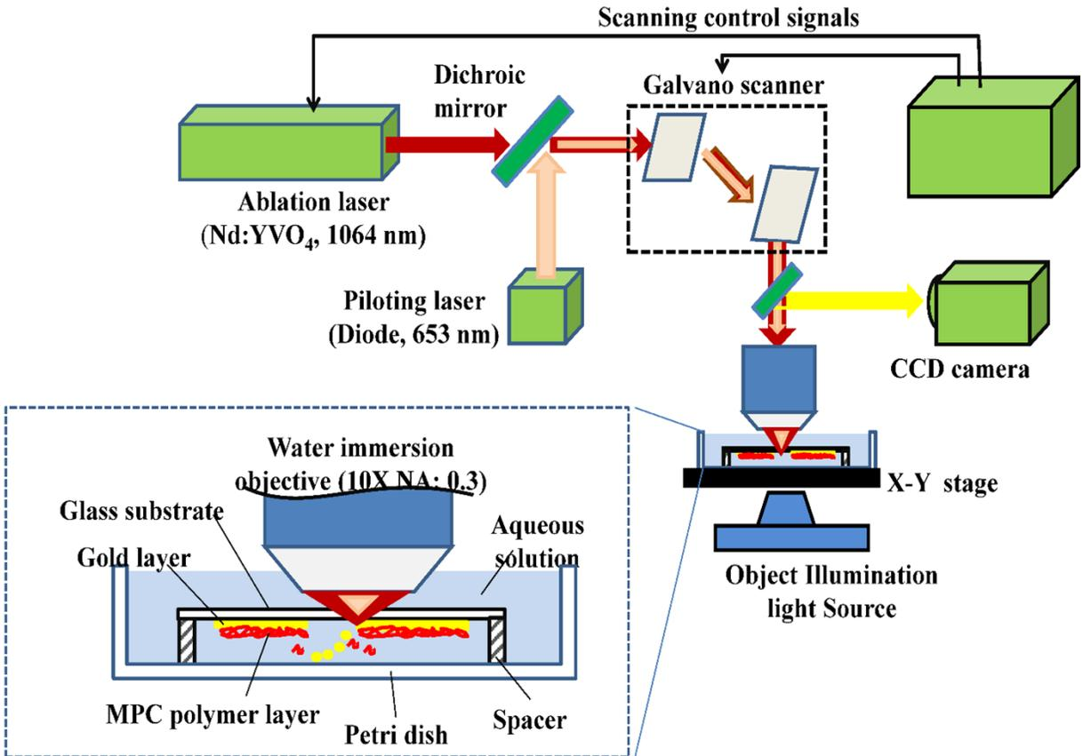
**Supplementary Fig. 1** Schematic diagram of laser fabrication setup. The system is designed to ablate the upper cytophobic layer on the substrate under physiologic aqueous conditions with high scanning rate.
