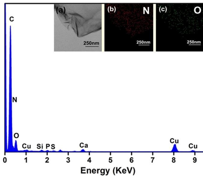
**Fig. S-3.** EDX spectrum of DNMG-1. (inset: TEM image of DNMG-1 (a), mapping of N (b) and mapping of O (c).)
