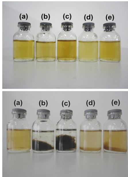
**Fig. S-7.** GO suspensions reduced by different components at 30°C for 5d in constant temperature incubator: (a) blank control with denitrifying medium only, (b) and (c) spent medium without cells, (d) and (e) cells only.
