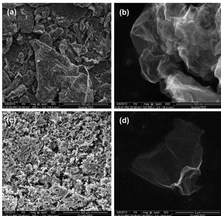
**Fig. S-4.** FESEM of images of (a  $\times 200$ , b  $\times 120\ 000$ ) CG and (c  $\times 200$ , d  $\times 30\ 000$ )
