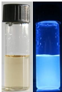
**Fig. S8** Photograph of 3-month N-CDs under illumination of white light (left) and UV (365 nm) light (right)
