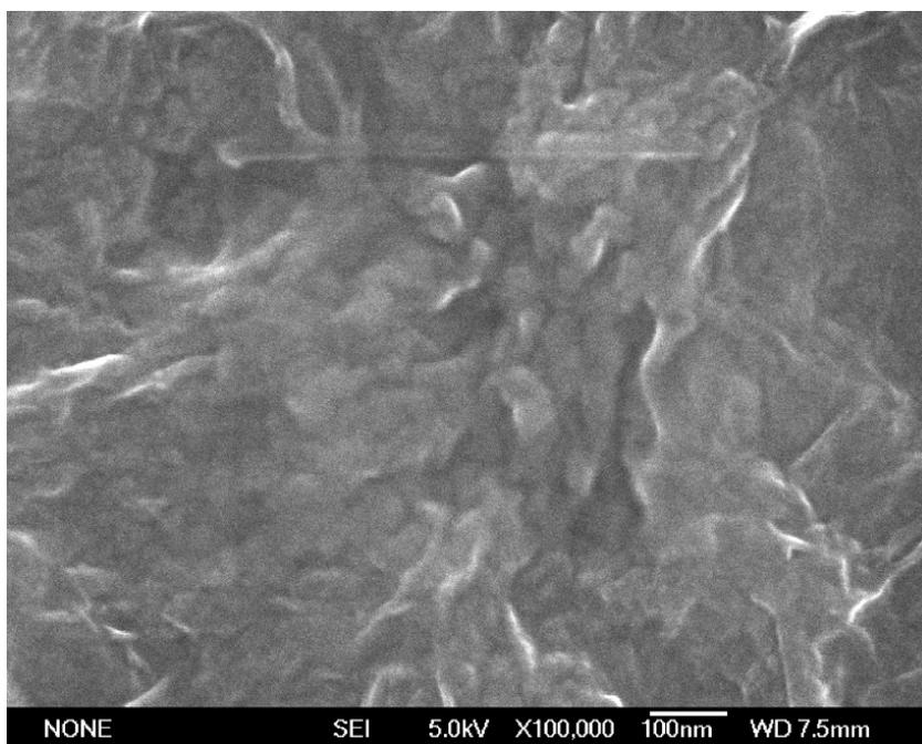
**Fig. S9** SEM image of N-CD/graphene.
