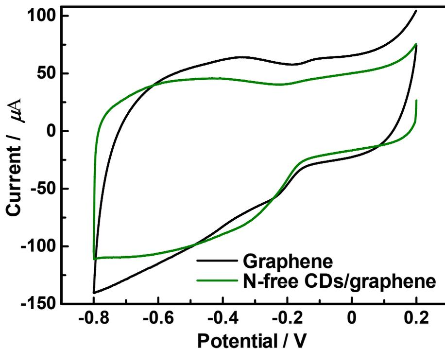
**Fig. S10** Cyclic voltammograms of hydrothermally treated graphene and N-free CDs/graphene on GC electrode in O<sub>2</sub>-saturated 1 M KOH.
