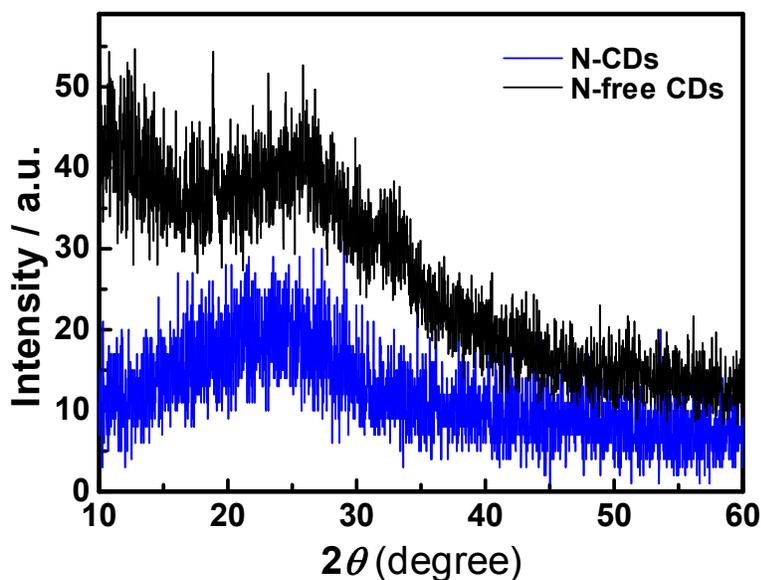
Fig. S1 XRD pattern of the as-prepared N-CDs and N-free CDs.
