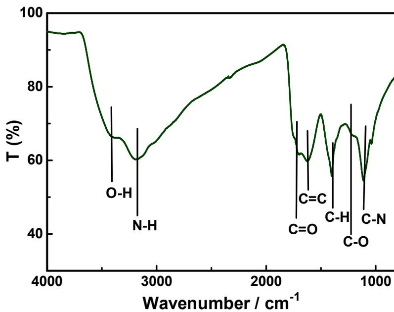
**Fig. S5** FTIR spectra of the obtained N-CDs.
