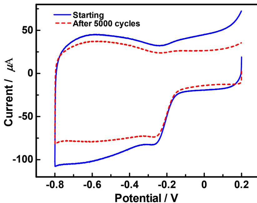
**Fig. S11** Electrochemical stability of N-CD/graphene as determined by continuous cyclic voltammetry in O<sub>2</sub>-saturated 1 M KOH.
