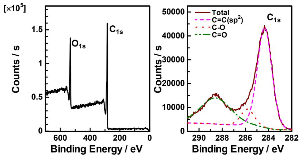
**Fig. S4** XPS spectrum (left) and high-resolution  $C_{1s}$  spectrum (right) of the N-free CDs.
