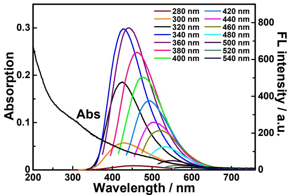
**Fig. S6** UV-Vis absorption and PL spectra (recorded for progressively longer excitation wavelengths in 20 nm increments) of the obtained N-free CDs.
