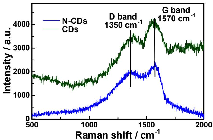
**Fig. S2** Raman spectra of the obtained N-CDs and N-free CDs.
