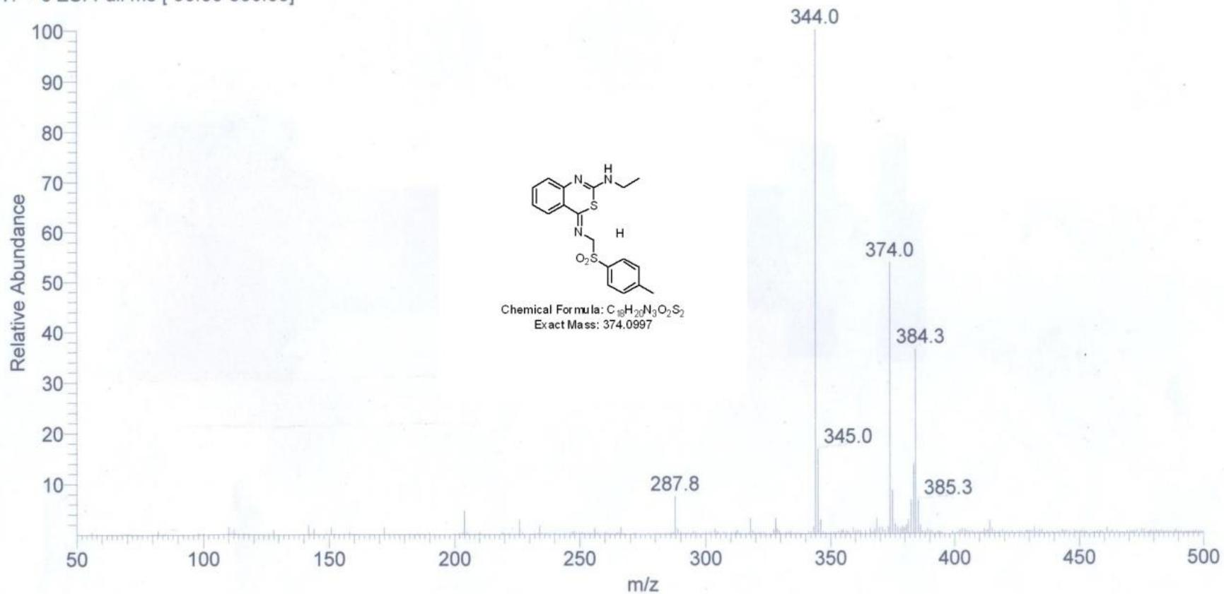
**Fig: S-55** ESMS spectra of (*Z*)-*N*-Ethyl-4-(phenylsulfonylmethylimino)-4*H*-benzo[*d*][1,3]thiazin-2-amine (**3fC**) (crude product)
