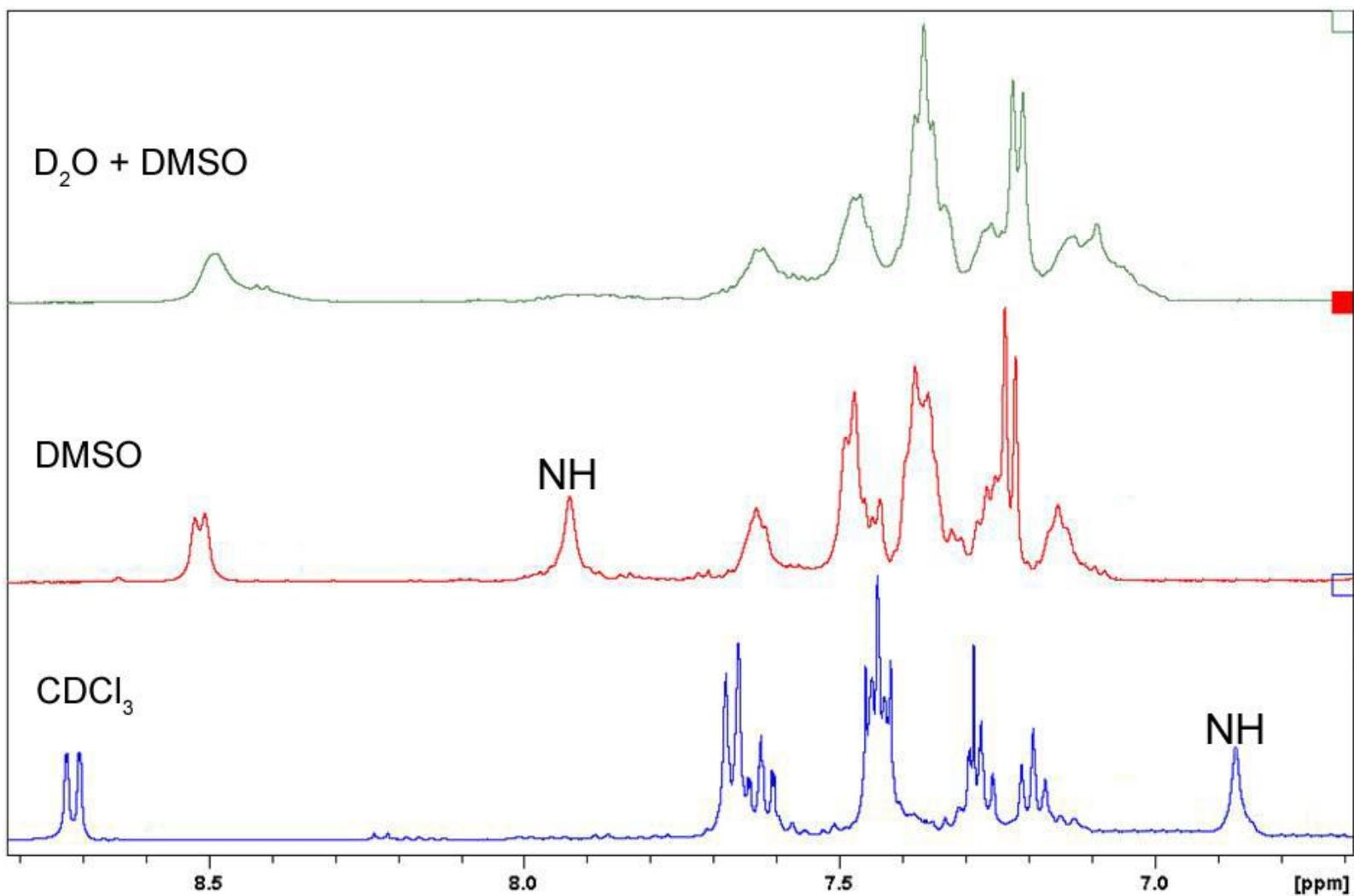
**Fig: S-3** Comparison between the <sup>1</sup>H spectra of (*Z*)-4-(Cyclohexylimino)-*N*-phenyl-4*H*-benzo[*d*][1,3]thiazin-2-amine (**3aA**) recorded in CDCl<sub>3</sub>, DMSO, D<sub>2</sub>O + DMSO for confirmation of the exocyclic NH group.
