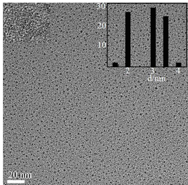
**Fig. S3** The TEM image of the GQDs derived from alcohol lamp soot by concentrated nitric acid oxidation. Insert: HRTEM (left) and the size distribution (right).
