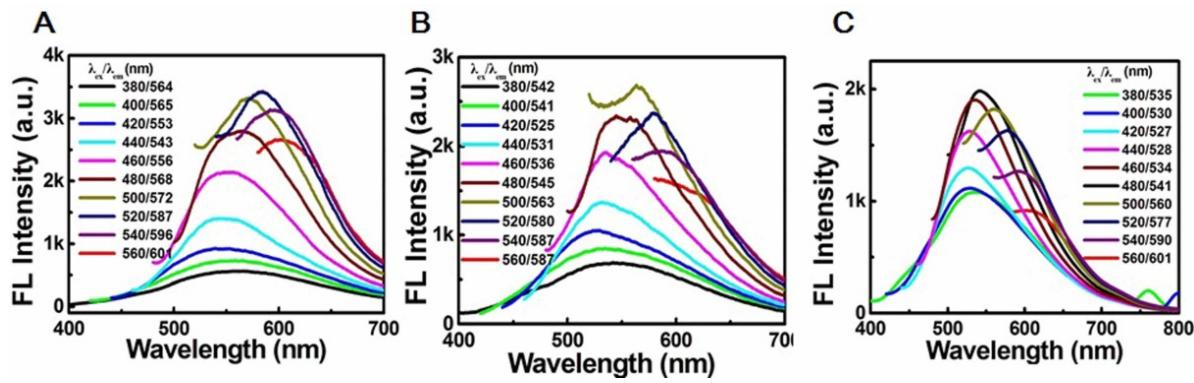
**Fig. S1** The fluorescence spectra of the GQDs synthesized by different concentration of nitric acid (reaction time is 3 h) at the excitation wavelengths from 380 nm to 560 nm in 20 increments. (A) 12 M, (B) 10 M, (C) 8 M, respectively.
