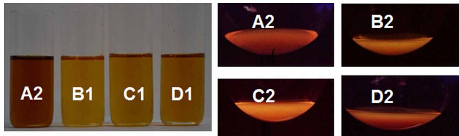
Fig. S5 The photographs of  $0.25 \text{ mg mL}^{-1}$  of the as-prepared GQDs under room light and UV light (365 nm) in *N*, *N*-dimethylformamide (A1, A2), water (B1, B2), alcohol (C1, C2), ethyl acetate (D1, D2), respectively.
