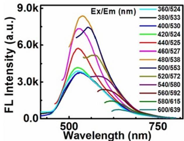
**Fig. S2** The fluorescence spectra of the GQDs derived from alcohol lamp soot by concentrated nitric acid oxidation.
