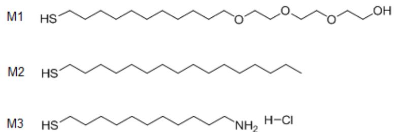
**Figure S2.** Chemical structures of thiol derivatives presenting tri(ethylene glycol) (EG<sub>3</sub>, M1), methyl (HDT, M2) and primary amine (NH<sub>2</sub>, M3) terminal groups used to form self-assembled monolayers (SAMs) on gold substrates.
