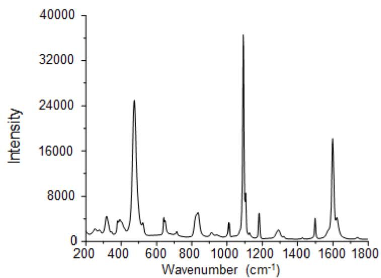
**Figure S9.** Raman spectrum of 4-ATP powder.
