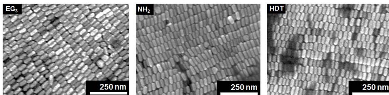
**Figure S3.** SEM images of ordered assemblies of gold nanorods on self-assembled monolayers (SAMs) presenting different functional groups such as EG<sub>3</sub>, NH<sub>2</sub> and HDT.
