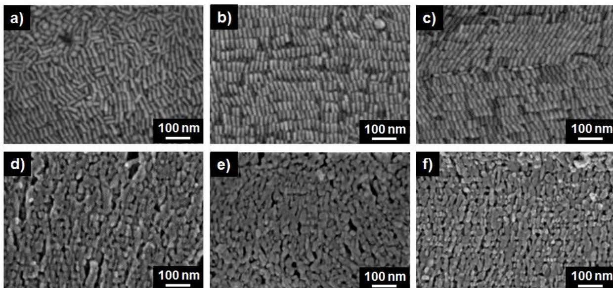
**Figure S7.** SEM images of ordered assemblies of GNRs on EG<sub>3</sub> (a), NH<sub>2</sub> (b) and HDT (c). SEM images of ordered assemblies of GNRs on EG<sub>3</sub> (d), NH<sub>2</sub> (e) and HDT (f) after 1 min piranha treatment.
