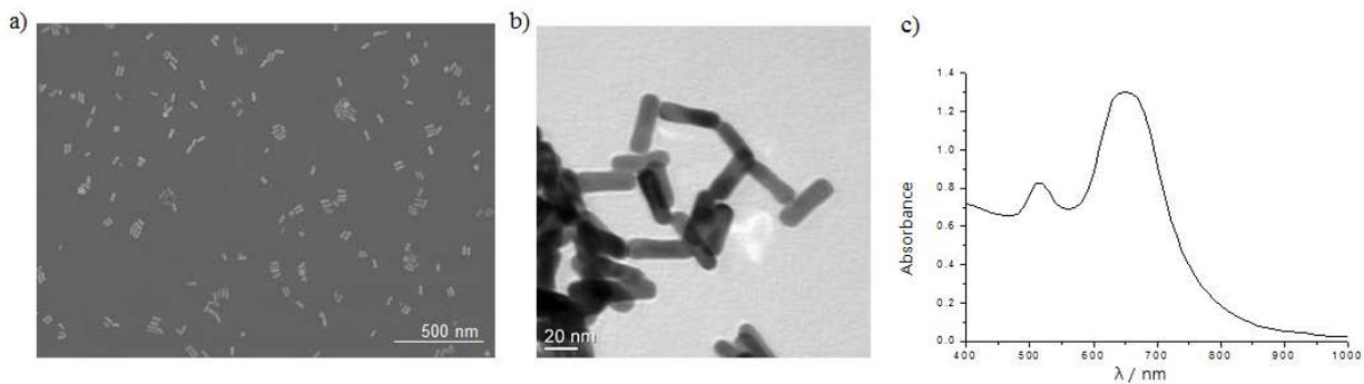
**Figure S1.** a) SEM and TEM (b) image. c) UV-vis absorption spectrum of the synthesized GNRs with an average diameter, length, aspect ratio of  $25 \pm 2$  nm,  $50 \pm 2$  nm and  $2.1 \pm 0.2$  and two specific surface plasmon bands at around 520 and 650 nm corresponding to short and long axis of GNRs.
