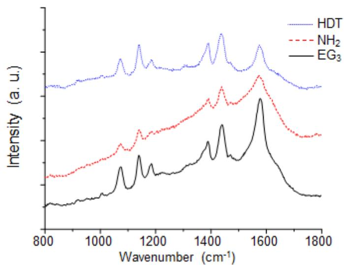
**Figure S8.** SERS spectra of 4-ATP from ordered assemblies of GNRs formed on SAMs presenting EG<sub>3</sub> (a), NH<sub>2</sub> (b) and HDT (c) without piranha treatment.
