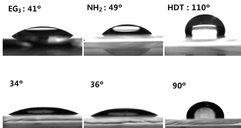
**Figure S6.** The contact angles of water (first row) and gold nanorod suspension (second row) on SAMs presenting different functional groups such as EG<sub>3</sub>, NH<sub>2</sub> and HDT.
