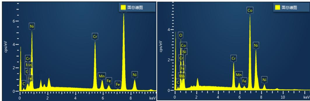
**Fig. S3** Energy-dispersive X-ray spectra of substrate (left) and  $\text{Co}_3\text{O}_4$  (right) grown on the substrate
