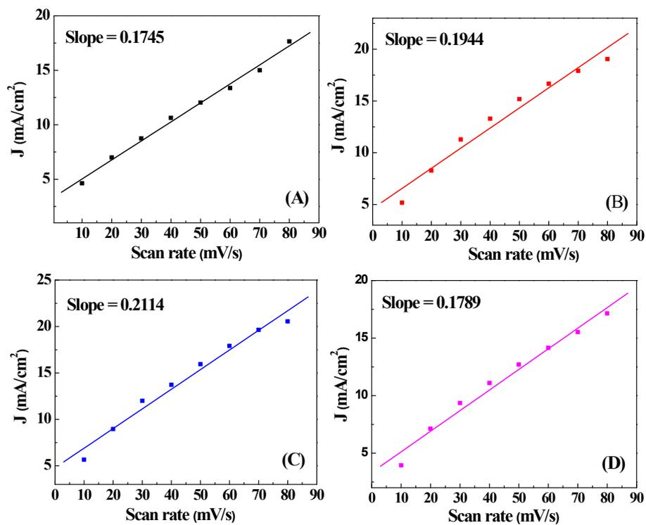
**Fig. S7** Linear relationship of the peak current density of  $\text{Co}^{3+}/\text{Co}^{2+}$  oxidation wave with the scan rate (A)  $\text{Co}_3\text{O}_4$ , (B)  $\text{Co}_3\text{O}_4$ -1, (C)  $\text{Co}_3\text{O}_4$ -3, (D)  $\text{Co}_3\text{O}_4$ -5 (tested in 0.1 M KOH)
