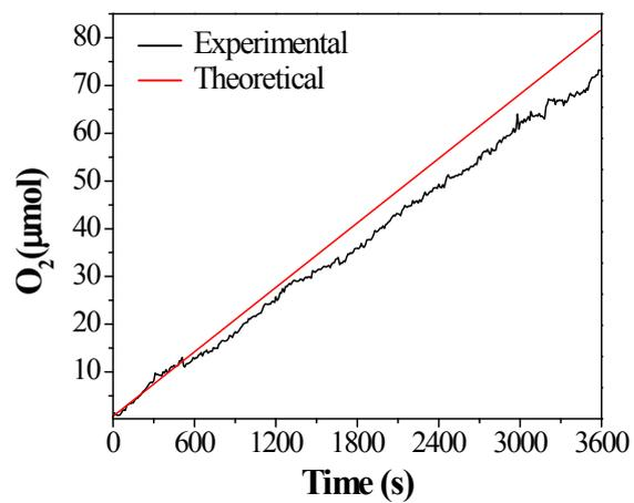
**Fig. S8** O<sub>2</sub> evolution measurements from the Co<sub>3</sub>O<sub>4</sub>-3 electrode using an O<sub>2</sub> probe method (at 1.64 V vs RHE)
