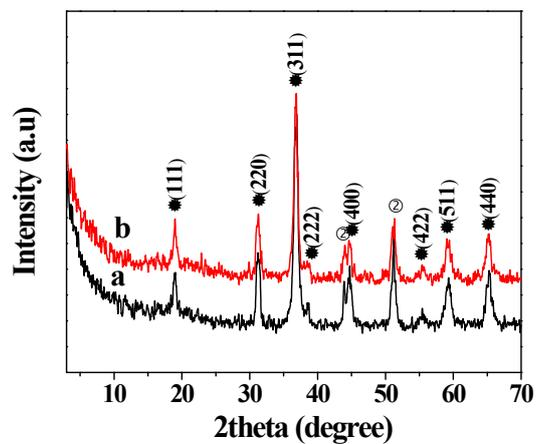
**Fig. S10** XRD pattern of Co<sub>3</sub>O<sub>4</sub>-3 electrocatalyst before OER (a) and after 12 hr OER operation (b) (triangle: reflections from Ni)
