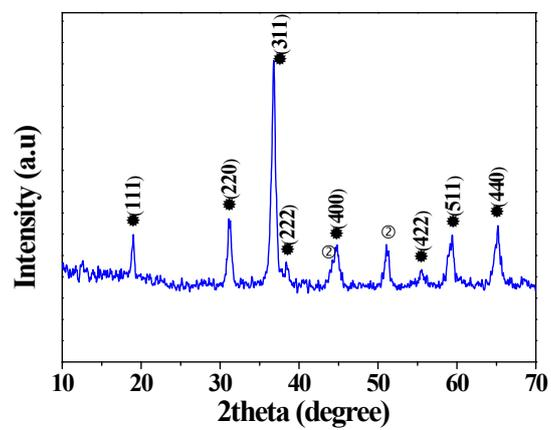
**Fig. S1** XRD pattern of  $\text{Co}_3\text{O}_4$ -NW grown on a Ni foil (triangle: reflections from Ni)
