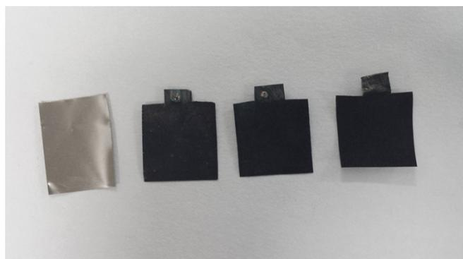
**Fig. S2** Digital photos of bare substrate,  $\text{Co}_3\text{O}_4$ ,  $\text{Co}_3\text{O}_4$ -3, and  $\text{Co}_3\text{O}_4$ -NW electrodes
