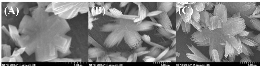
**Fig. S9** SEM images of Co<sub>3</sub>O<sub>4</sub> samples after 12 hr OER operation (1.58 V, 0.1 M KOH). (A) Co<sub>3</sub>O<sub>4</sub>, (B) Co<sub>3</sub>O<sub>4</sub>-1, (C) Co<sub>3</sub>O<sub>4</sub>-5
