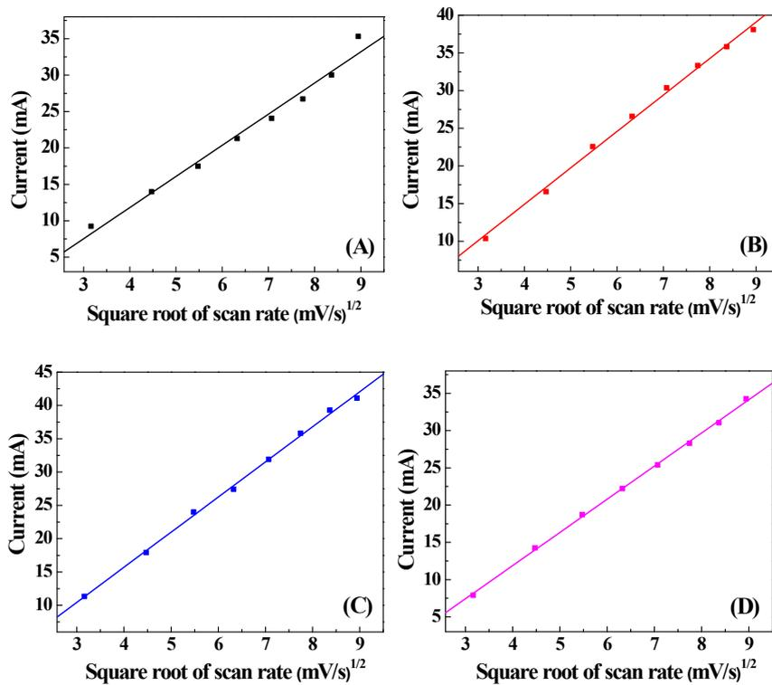
**Fig. S5** Linear dependence of the peak current of the  $\text{Co}^{3+}/\text{Co}^{2+}$  oxidation wave with the square root of scan rate (A)  $\text{Co}_3\text{O}_4$ , (B)  $\text{Co}_3\text{O}_4-1$ , (C)  $\text{Co}_3\text{O}_4-3$ , (D)  $\text{Co}_3\text{O}_4-5$  (tested in 0.1 M KOH)
