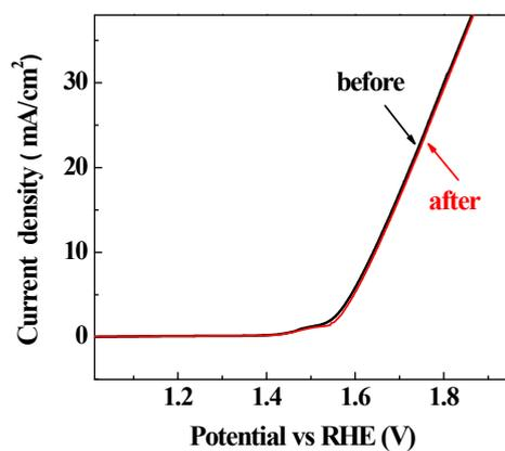
**Fig. S11** LSV curves of Co<sub>3</sub>O<sub>4</sub>-3 electrocatalyst before OER (black) and after 12 hr OER operation (red) (1.58 V vs RHE, 0.1 M KOH)
