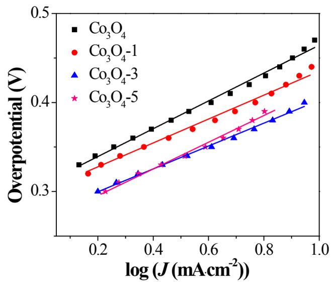
**Fig. S6** Tafel plots of  $\text{Co}_3\text{O}_4$  electrodes. The Tafel slopes were derived by fitting data in the linear part of the plots.
