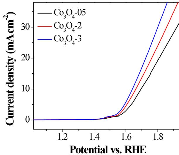
**Fig. S4** Linear sweep voltammetry (LSV) curves of  $\text{Co}_3\text{O}_4$  electrodes treated with different amount of solute (tested in 0.1 M KOH):  $\text{Co}_3\text{O}_4$ -05 (0.5wt%),  $\text{Co}_3\text{O}_4$ -2 (2wt%),  $\text{Co}_3\text{O}_4$ -3 (3wt%).
