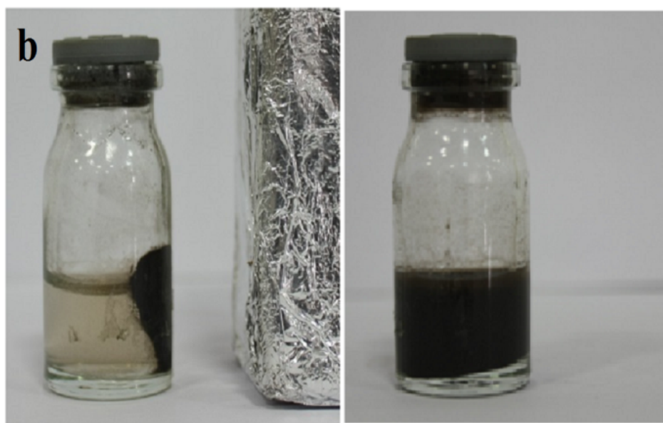
Figure 4. a) The VSM of AGu@MGO nanosheets, and b) magnetic separation of Pd@AGu@MGO nanosheets.
