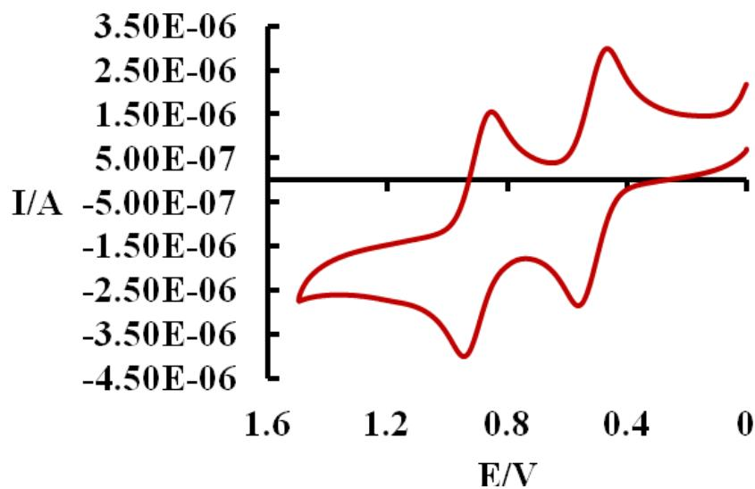
**Figure S68:** Cyclic voltammogram (CV) for **6b** (DCM, electrolyte TBAPF<sub>6</sub>; working electrode: Pt; ref. electrode: Ag/AgCl; Scan rate 100 mV s<sup>-1</sup>).
