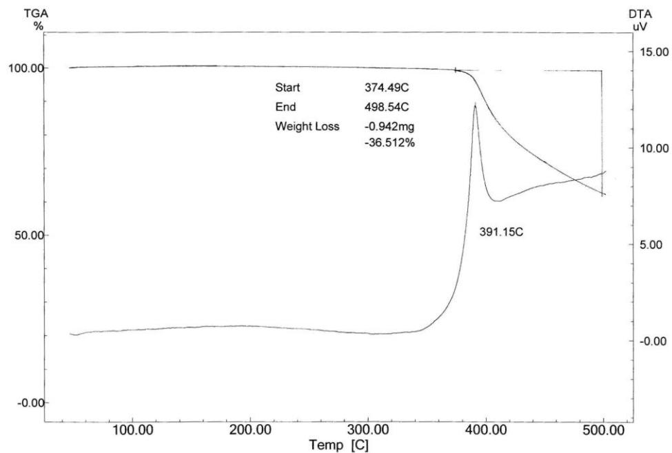
**Figure S71:** TGA Analysis of **6b** under N<sub>2</sub> with temperature rise of 10°C per minute. **6b** is highly stable as it is having a high thermal decomposition temp. of about >391°C.
