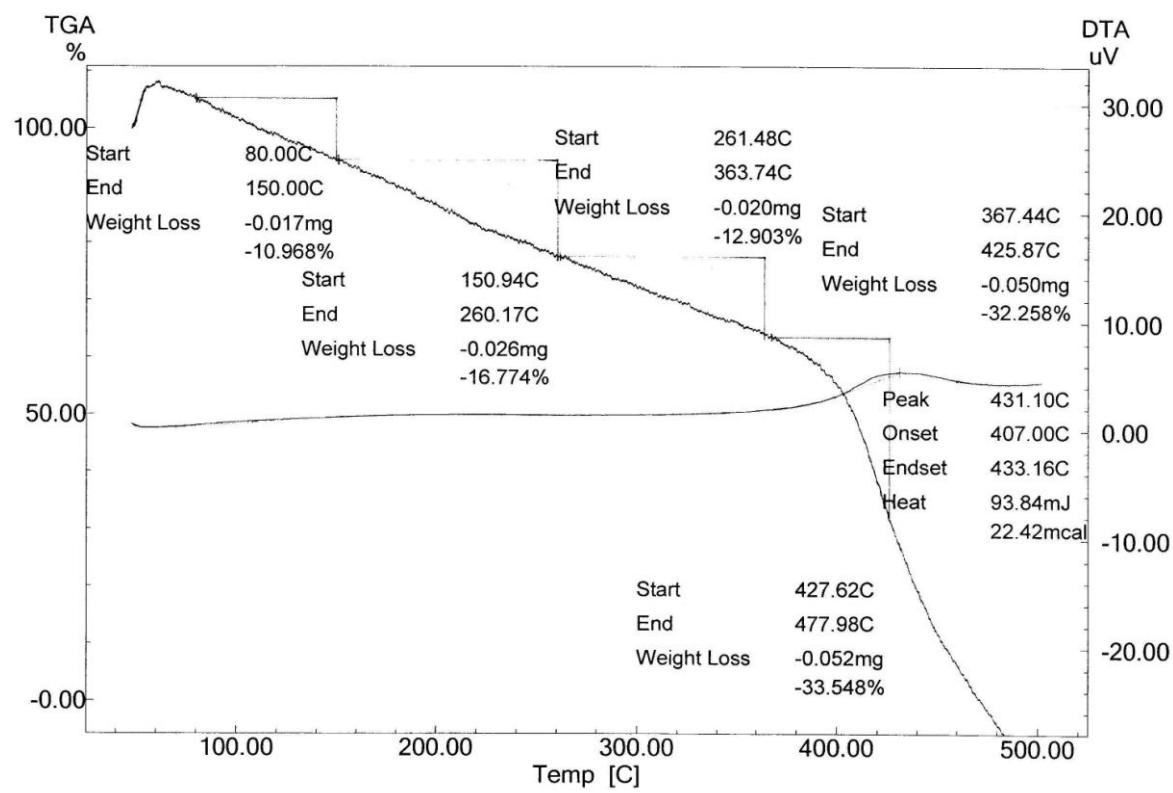
**Figure S72:** TGA Analysis of **6c** under N<sub>2</sub> with temperature rise of 10°C per minute. **6c** is highly stable as it is having a high thermal decomposition temp. of about >407°C.
