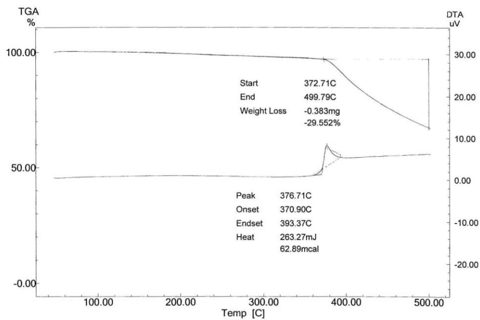
**Figure S70:** TGA Analysis of **6a** under N<sub>2</sub> with temperature rise of 10°C per minute. **6a** is highly stable as it is having a high thermal decomposition temp. of about >371°C.
