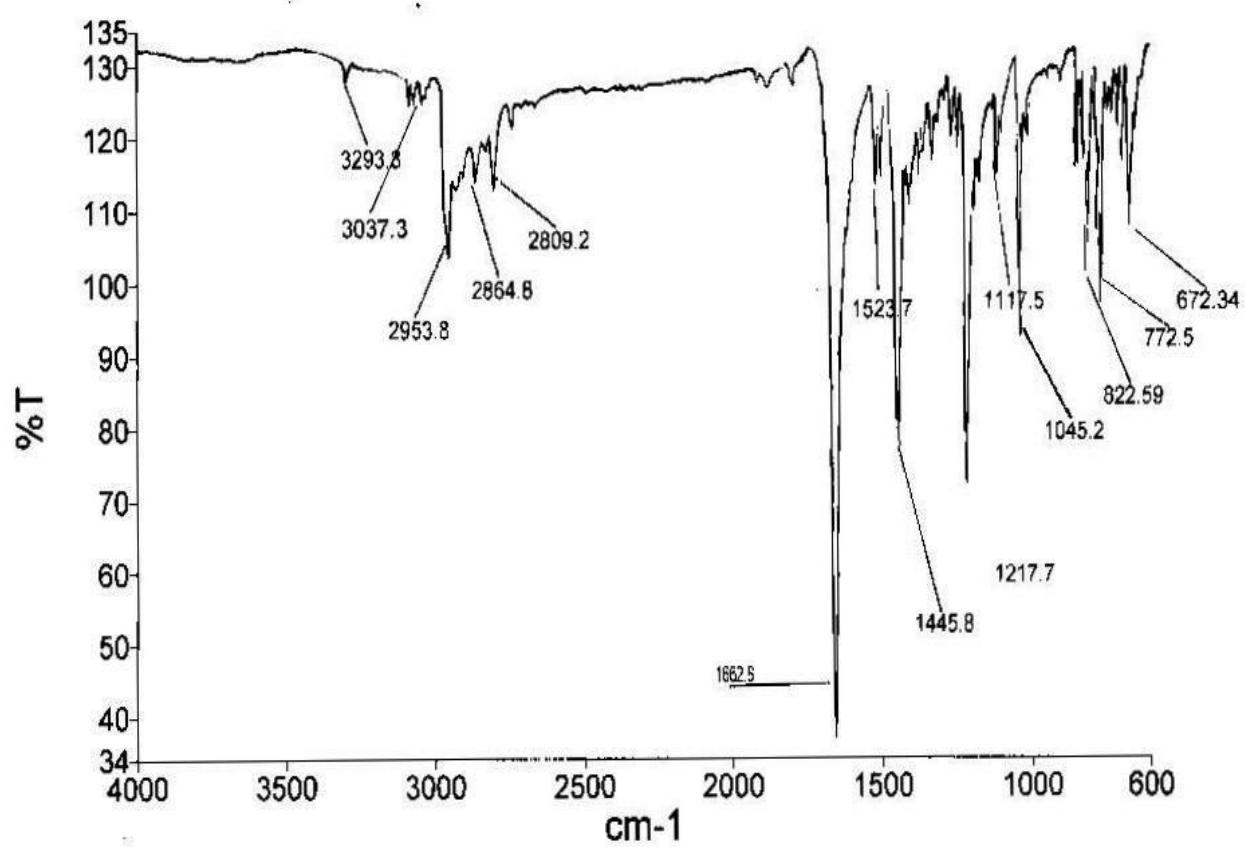
Figure S24: IR Spectrum of 4c.
