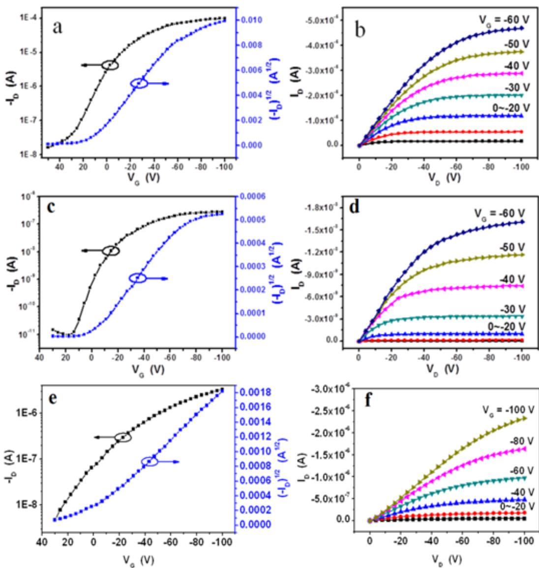
**Figure S73:** Typical transfer (a) and output (b) characteristics of FET devices based on **6a**, with OTS-treated SiO<sub>2</sub>/Si substrate ( $T_s = 100$  °C). Typical transfer (c) and output (d) characteristics of FET devices based on **6b**, with OTS-treated SiO<sub>2</sub>/Si substrate ( $T_s = 25$  °C). Typical transfer (e) and output (f) characteristics of FET devices based on **6c**, with OTS-treated SiO<sub>2</sub>/Si substrate ( $T_s = 25$  °C).
