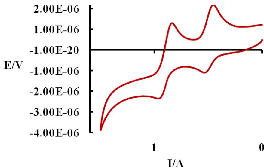
**Figure S69:** Cyclic voltammogram (CV) for **6c** (DCM, electrolyte TBAPF<sub>6</sub>; working electrode: Pt; ref. electrode: Ag/AgCl; Scan rate 100 mV s<sup>-1</sup>).
