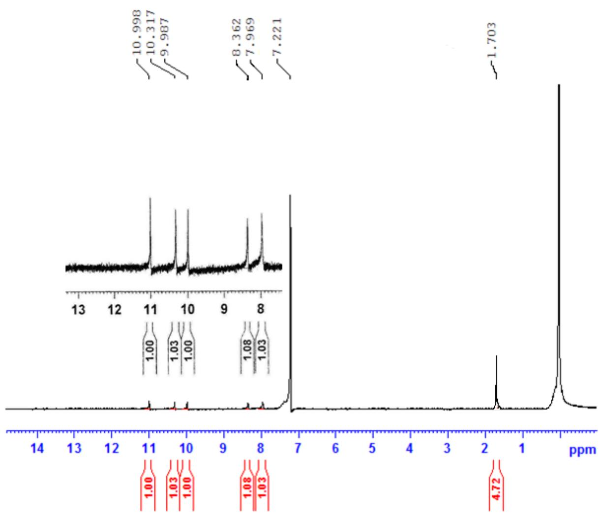
Figure S45: <sup>1</sup>H NMR Spectrum of 6c.
