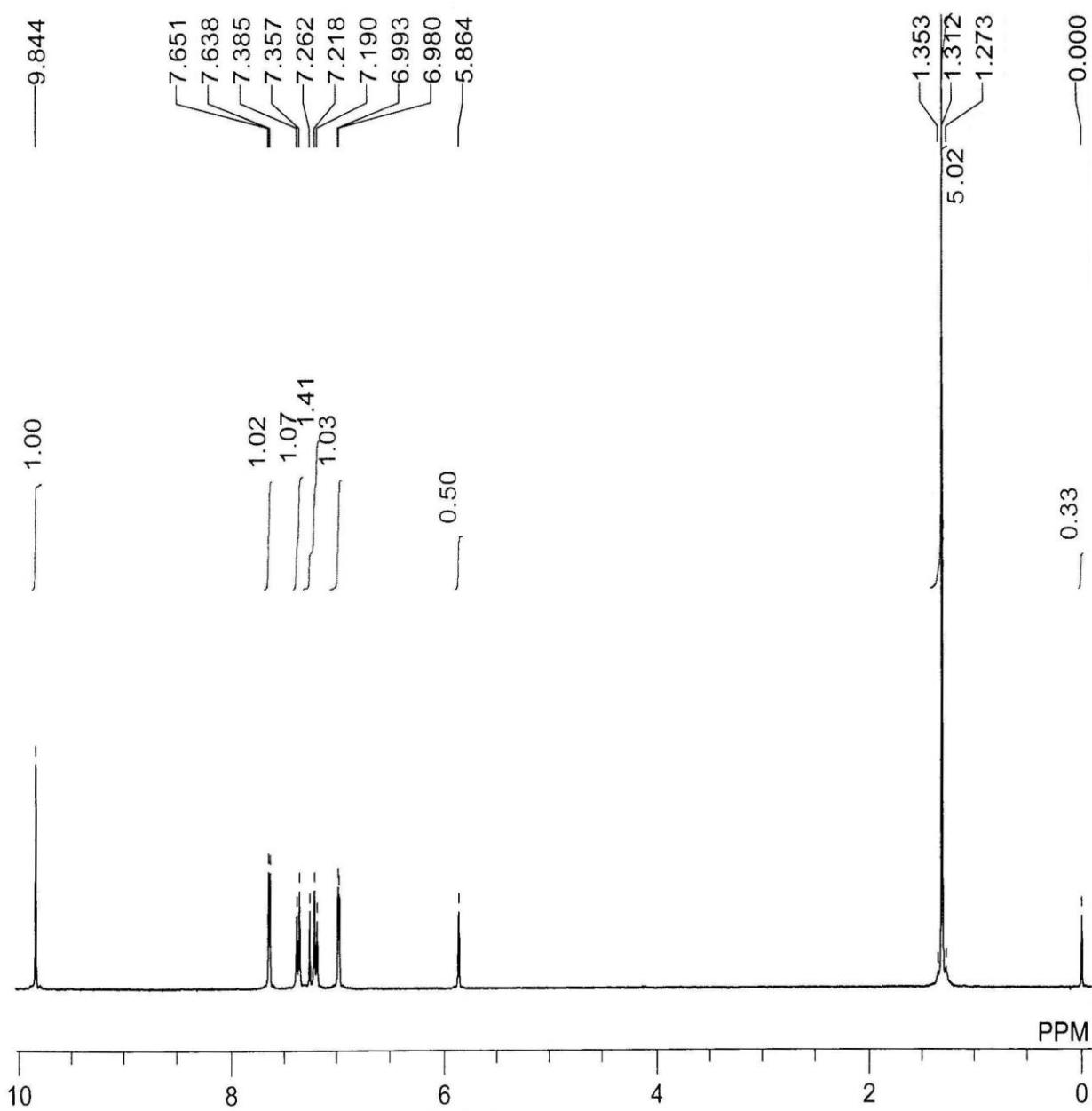
Figure S21:  $^1\text{H}$  NMR Spectrum of 4c.
