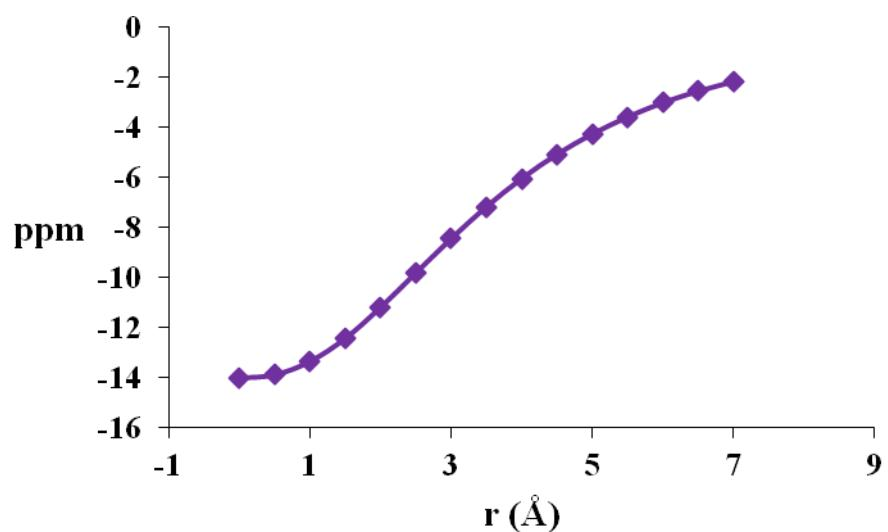
**Figure S55:** The ghost (Bq) atoms (in purple) were placed (0.5 Å interval) in the centre of **6c**. The -ve NICS values clearly indicate the aromaticity of **6c**. NICS is maximum at 0 Å and decreases as the distance of the ghost atom is increased in 0.5 Å intervals.
