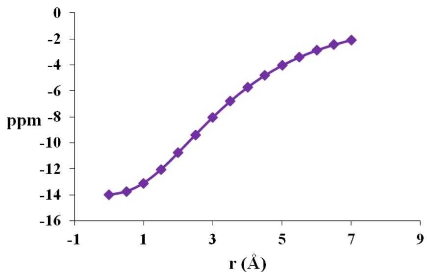
**Figure S52:** The ghost (Bq) atoms were placed (0.5 Å interval) in the centre of the molecule (in purple). The -ve NICS values clearly indicate the aromaticity of **6b**. NICS is maximum at 0 Å and decreases as the distance of the ghost atoms is increased in 0.5 Å intervals.
