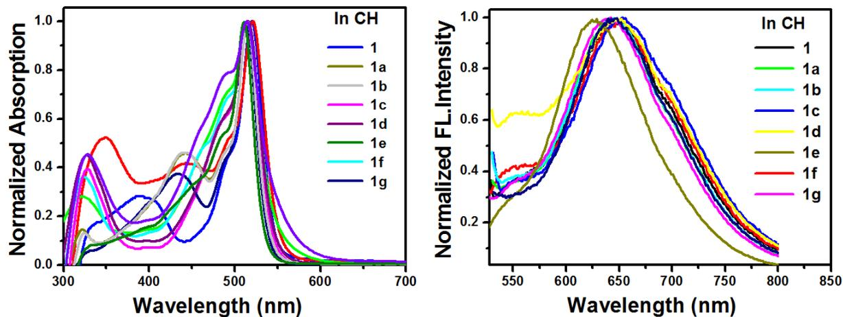
**Fig 15:** Normalized absorption and fluorescence (FL) emission spectra of BODIPY dyes **1**, **1a-1g** in cyclohexane (CH).
