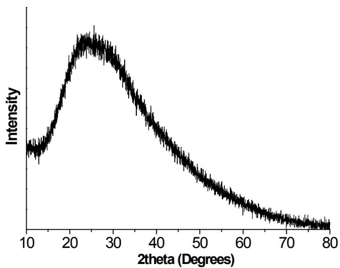
Fig. S2. XRD spectrum of CDs with one broad peak centered at  $2\theta=25^\circ$ .
