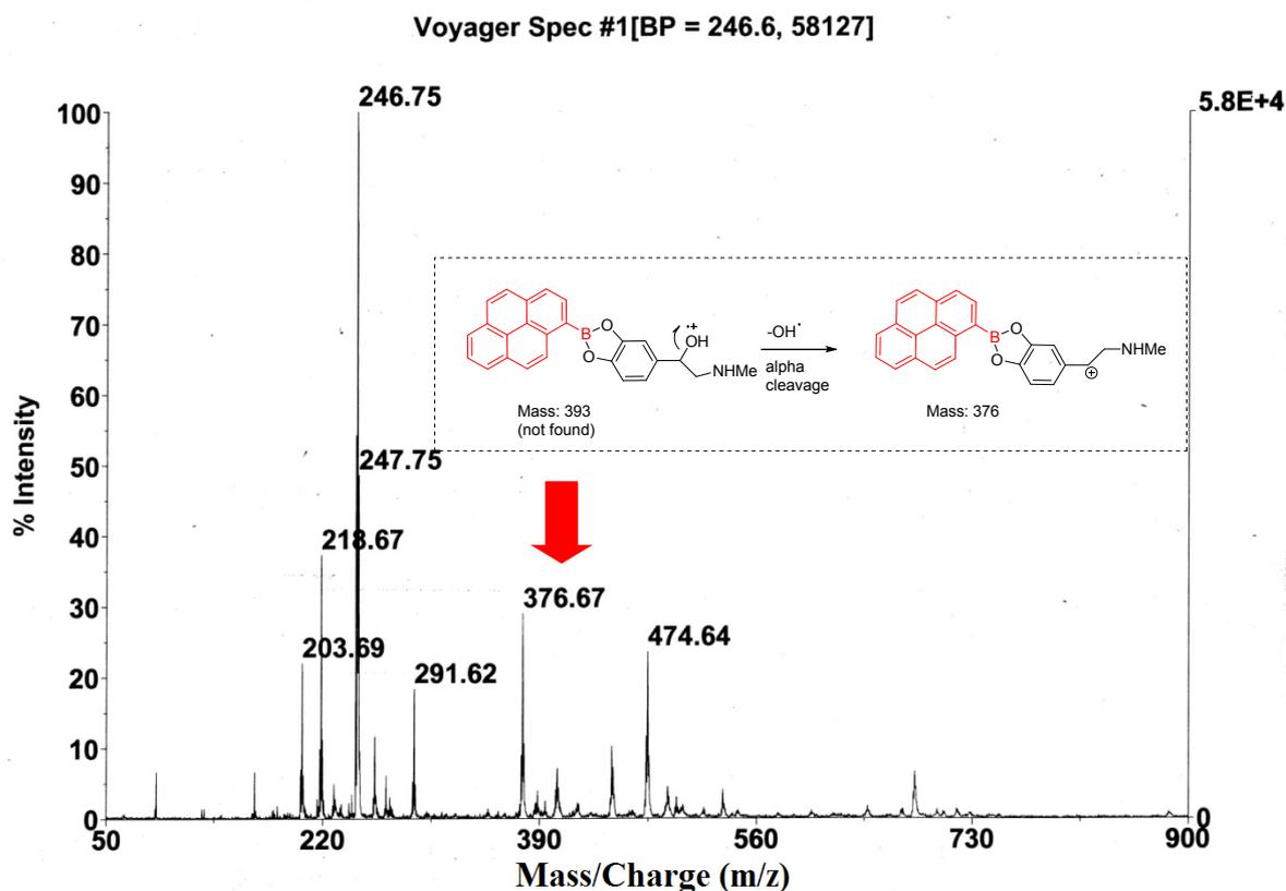
Fig: LA-LDI-TOF Mass Spectrum of epinephrine (+ve ion mode)
