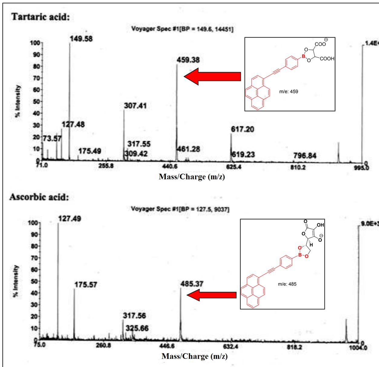
**Fig:** LA-LDI spectrum of the synthesised probe with Tartaric and ascorbic acid (Both the spectra were recorded in **negative ion mode**. The spectra are much clean compare to PBA complexes).
