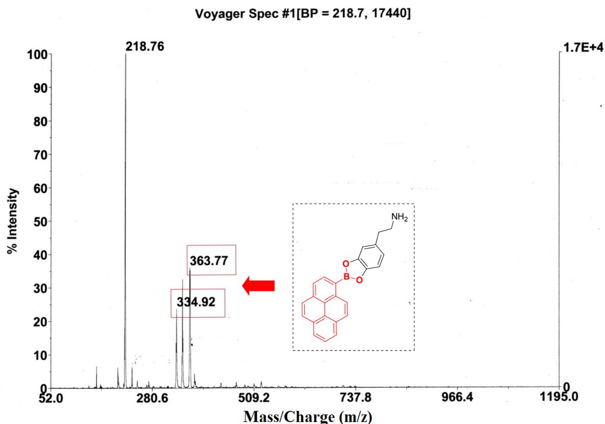
**Fig:** LA-LDI-TOF Mass Spectrum of dopamine (+ve ion mode)
