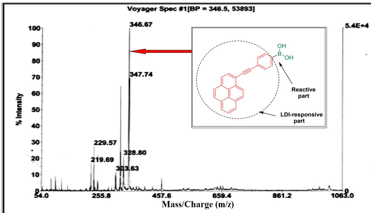
Fig: LA-LDI spectrum of the synthesised probe (+ve ion mode).
