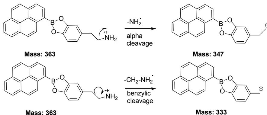
Fig: Schematic diagram showing the generation of different ion fragments from PBA-DA complex
