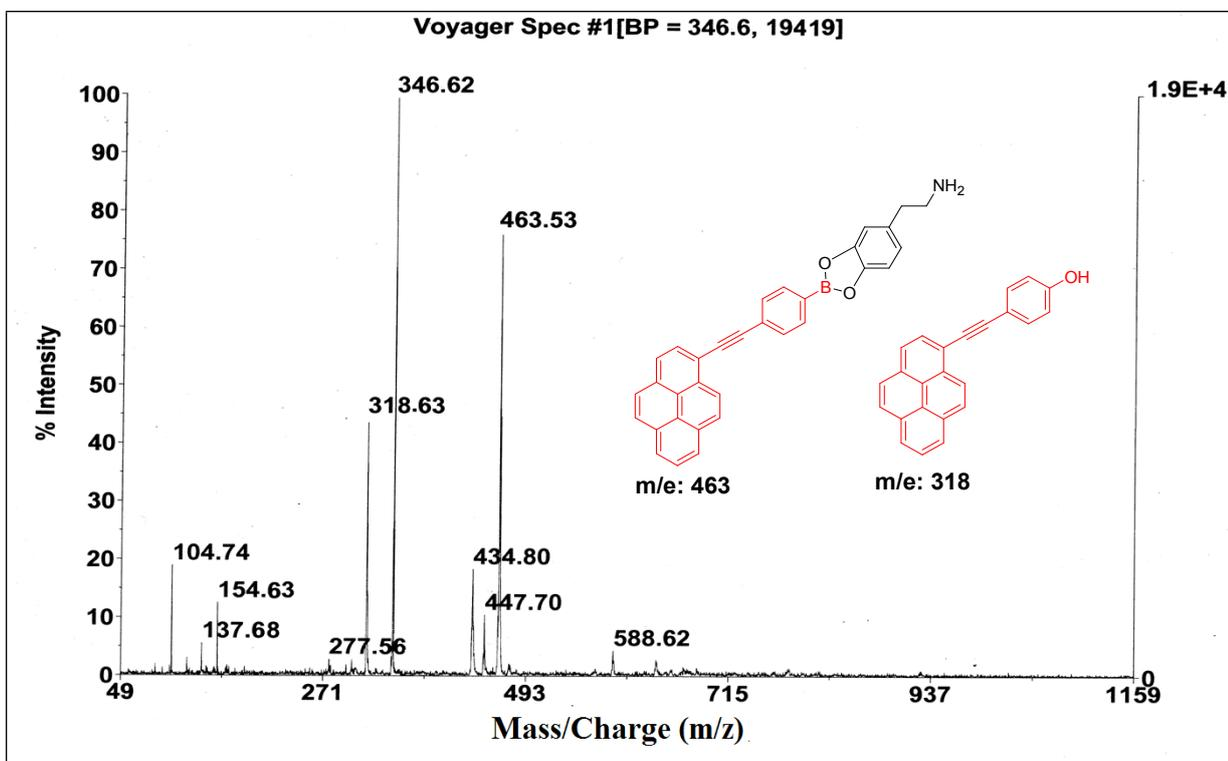
Fig: LA-LDI spectrum of the synthesised probe and Dopamine complex (+ve ion mode, Intensity is much higher).
