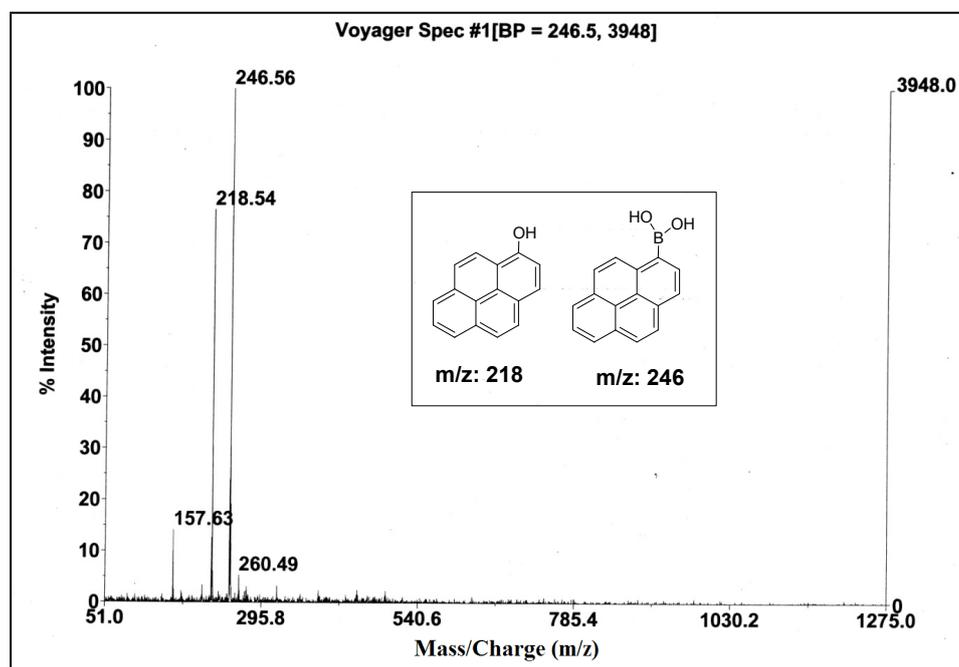
Formation of different species from pyrene-1-boronic acid during acquisition of mass spectra is shown as follows (*Ar*: pyrene):
