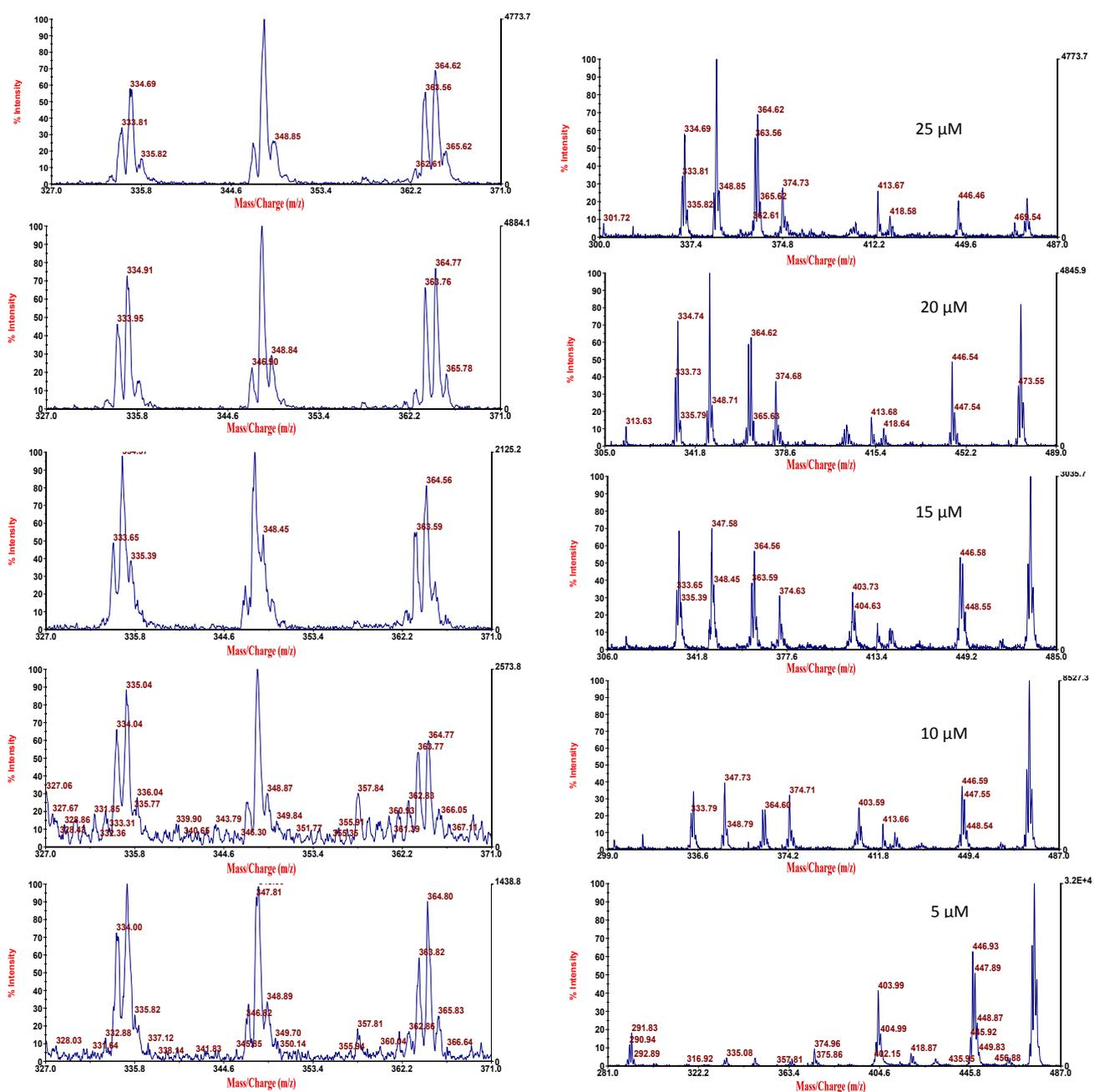
Fig: Concentration dependent variation of intensities of peaks for dopamine at  $m/z$  363,  $m/z$  347 and  $m/z$  334 (Left panel is showing variation of dopamine complex. 2.Right panel is showing relative variation of dopamine complex with respect to boronic acid derivative).
