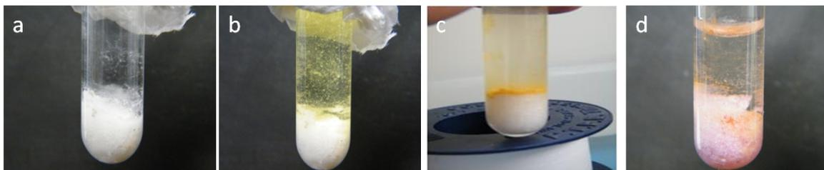
Fig. S3: (a) The freshly prepared gel of **6** (DMF/water, 5%, w/v) , (b) aqueous solution of  $\text{HAuCl}_4 \cdot x\text{H}_2\text{O}$  on the gel bed (photographed instantly), (c) the same solution on the gel bed after few hours ,(d) after 12 hours.
