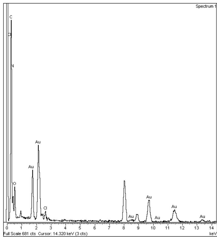
Fig. S2: EDX spectrum of Au nanoparticles on gel.
