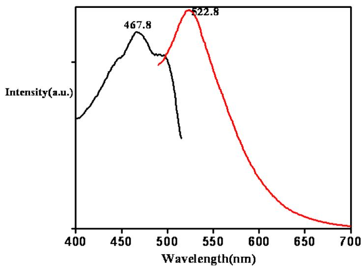
Fig. S14: Excitation (467.8nm) and emission spectrum (522.8nm) of AuNCs.
