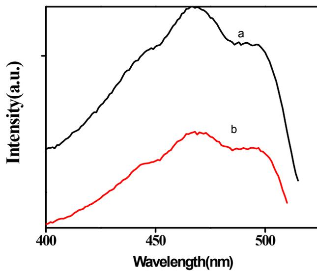
Fig. S13: Excitation spectrum of AuNCs (a) in absence and (b) in presence of Hg(II) ( $\lambda_{\text{em}} = 525\text{nm}$ ).
