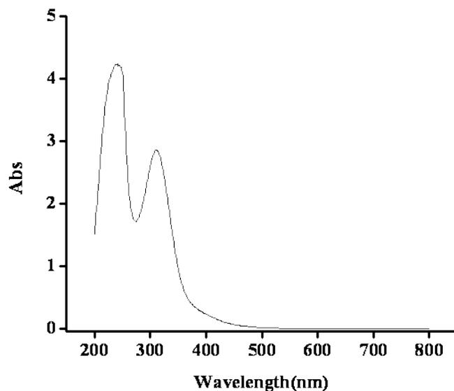
Fig. S7: UV-Vis spectrum of  $\text{H[AuCl}_4\text{]} \cdot x\text{H}_2\text{O}$  dissolved in Ethylene Glycol solvent, recorded after 48 hrs. No surface plasmon band indicating no formation of AuNPs.
