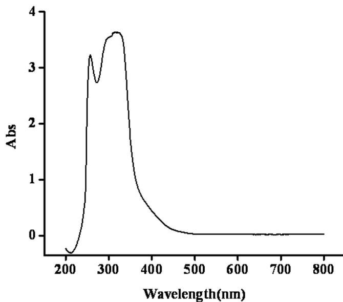
Fig. S6: UV-Vis spectrum of  $\text{H[AuCl}_4] \cdot x \text{H}_2\text{O}$  dissolved in DMF solvent, recorded after 48 hrs. There is no surface plasmon band, indicative of no formation of AuNPs.
