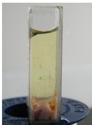
Fig. S4: Aqueous alkaline p-Nitrophenol (p-Nitrophenolate) solution kept on AuNP- embedded gel prepared from gelator **6** [DMF, water ; 5% (w/v)]; generated inside standard UV-Vis cell, in order to facilitate the monitoring of the p-Nitrophenolate  $\rightarrow$  p-Aminophenolate conversion by UV-Vis spectroscopy.
