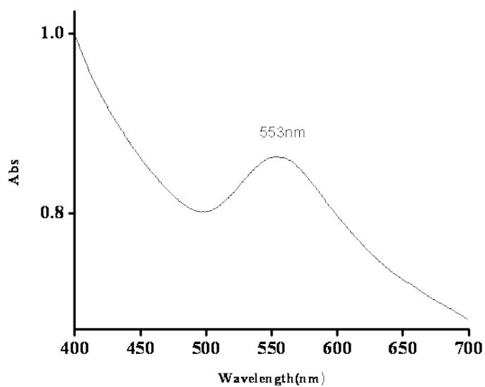
Fig. S8: UV-Vis spectrum of AuNPs generated on the gel bed of **6** (DMF/water medium), showing the surface plasmon band at 553nm.
