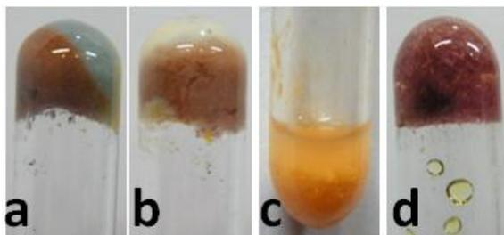
Fig. S5: Different colors of AuNPs; a) within a gel (DMF, water; 5%, w/v) of **1**; b) within a gel (DMF, water; 5%, w/v) of **5**; c) AuNP formed within a precipitate obtained from heated solution of gelator **6** in DMF and subsequent addition of water; d) within a gel (DMF, water; 5%, w/v) of **4**.
