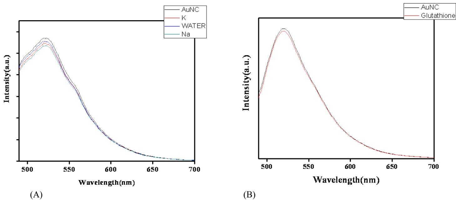
Fig. S15: The emission spectrum of AuNCs in presence of large excess of (A) NaCl (0.1 M), KCl (0.1 M) and water and (B) glutathione. The fluorescence response was found to be very stable.
