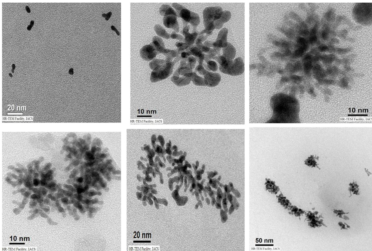
Fig.S9: Highly branched Au-nanodendrites formed when a DMF solution containing the gelators **2** or **6** was heated with  $\text{HAuCl}_4 \cdot x\text{H}_2\text{O}$ ; without any addition of water.
