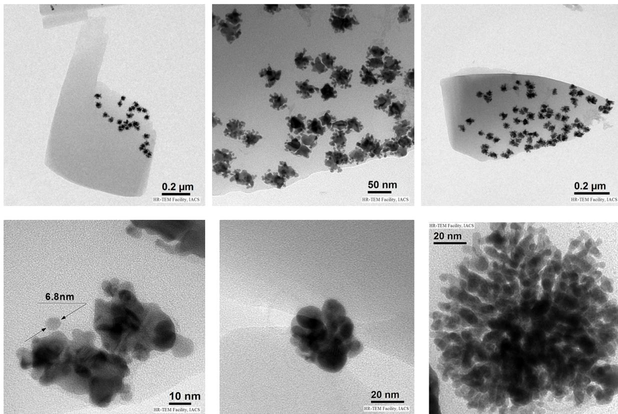
Fig.S10: Highly branched Au-nanodendrites formed in supramolecular gel of **2** (5% (w/v); DMF/water, 1:5 (v/v)).
