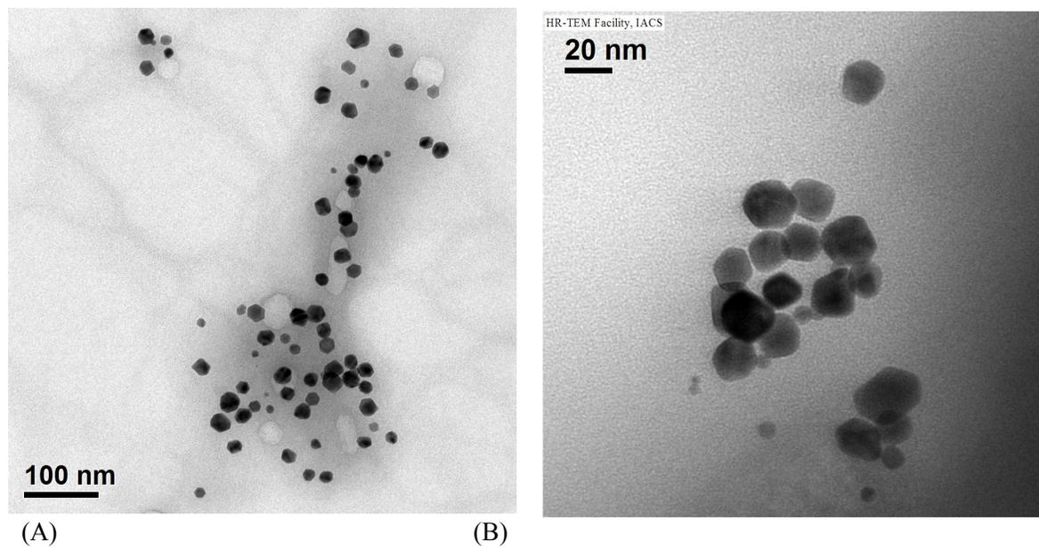
Fig. S11: Nanoparticles of different but regular shapes on gels derived from gelators (A) **5** and (B) **6** (5% (w/v), DMF:water, 1:5 (v/v)).
