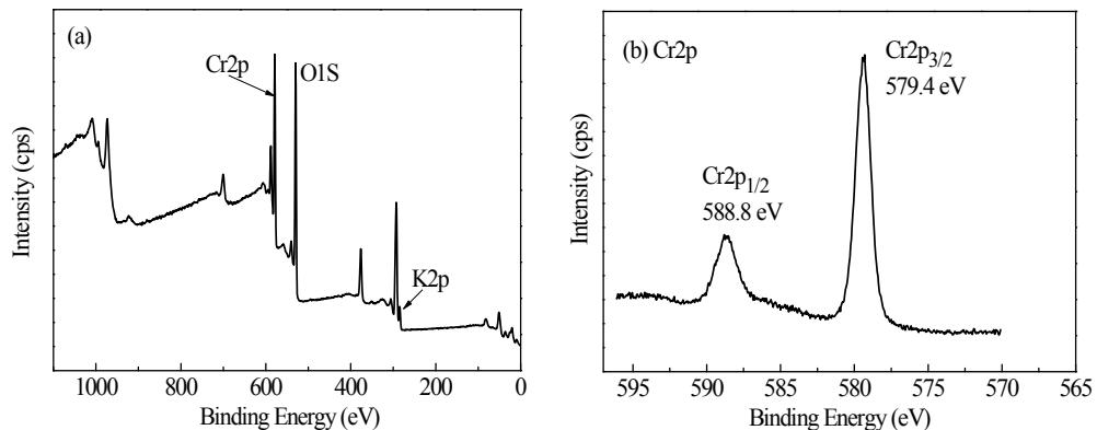
Fig. S4 (a) Survey XPS spectrum of  $\text{K}_2\text{Cr}_2\text{O}_7$  and (b) HR-XPS spectrum of Cr2p in  $\text{K}_2\text{Cr}_2\text{O}_7$ .
