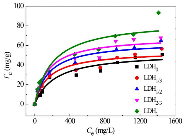
Fig. S3 Nonlinear correlation plots of Langmuir isotherm for Cr(VI) sorption onto Mg-Al-Fe LDHs
