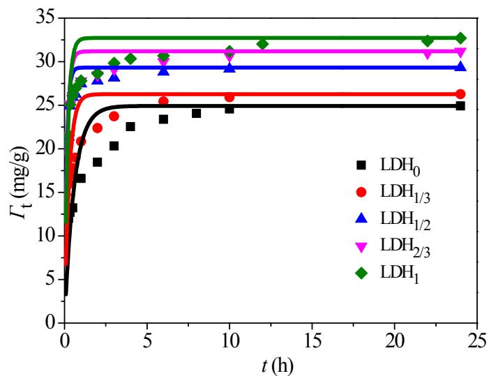
Fig. S2 Nonlinear correlation plots of pseudo first-order kinetics for Cr(VI) sorption onto Mg-Al-Fe LDHs.
