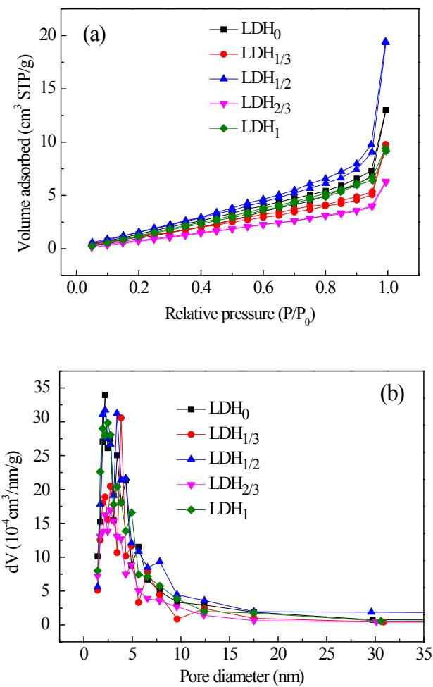
Fig. S1 (a) Nitrogen adsorption-desorption isotherms and (b) pore size distribution curves of Mg-Al-Fe LDHs samples.<sup>†</sup>
