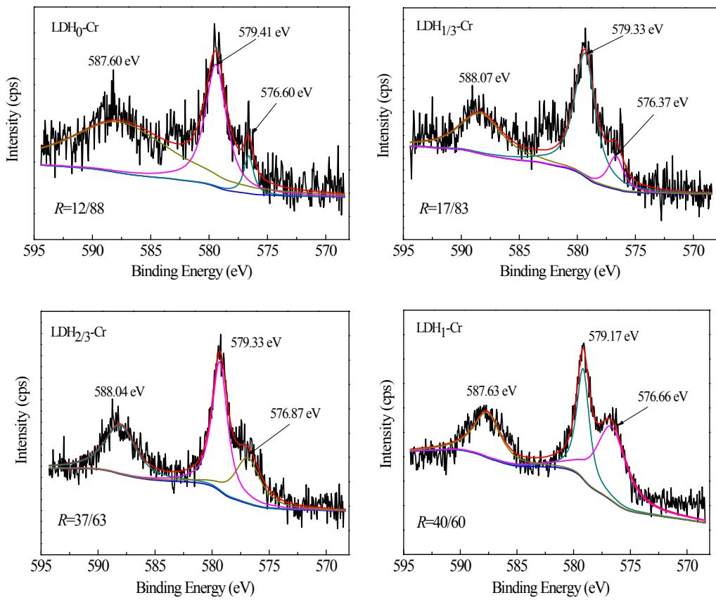
Fig. S6 HR-XPS spectra of Cr 2p for various LDHs-Cr samples. The  $R$  value in each figure is the area ratio of the peak about at  $E_B$  576 eV to the peak about at  $E_B$  579 eV.
