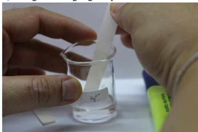
4) dipping in an aqueous solution of  $\text{Hg}^{2+}$
