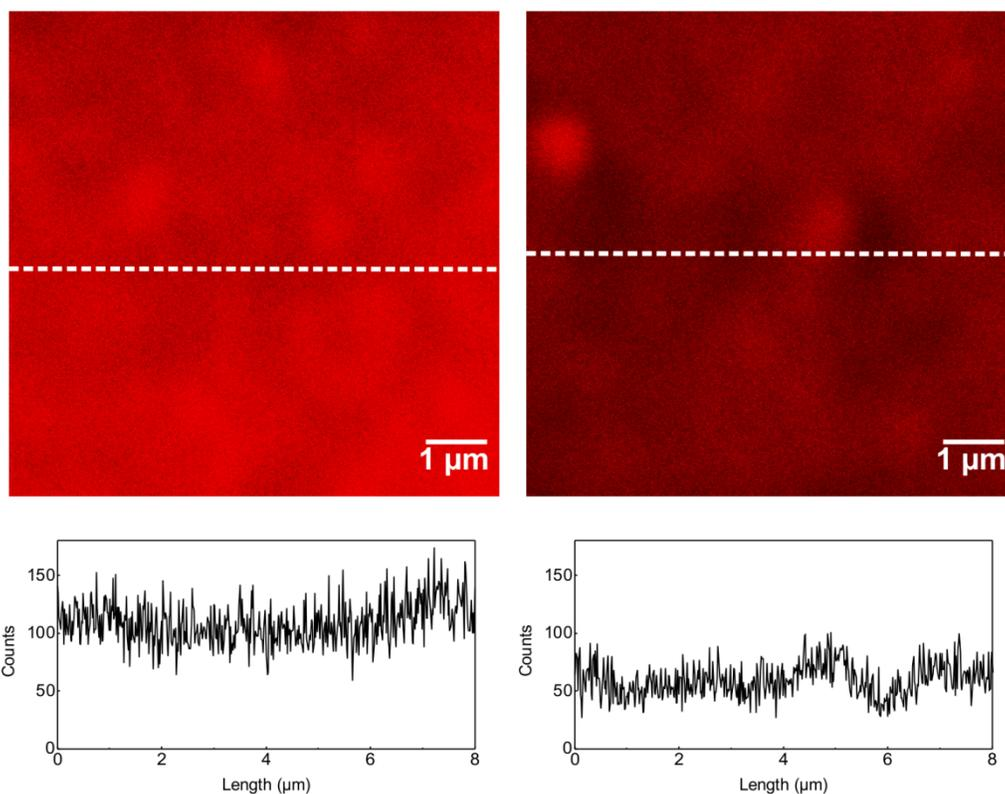
Figure S5. Laser scanning confocal microscopy images and fluorescence counts of patterned PDMAEMA brushes after protein adsorption (left) and after protein desorption (right). The average fluorescence counts decrease to ~47% of the original counts, indicating that ~53% BSA is released from the polymer brushes.
