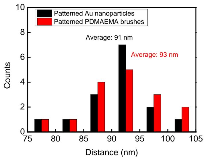
Figure S1. Statistical analysis of distance between neighboring Au nanoparticles and patterned PDMAEMA brushes. The AFM height images of the two samples are shown in Figure 1 in the main text.
