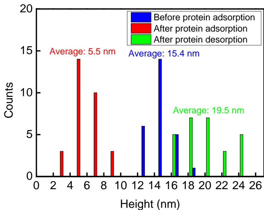
Figure S7. Statistical analysis of height of patterned PDMAEMA brushes before protein adsorption (blue), after protein adsorption (red), and after protein desorption (green). The AFM topography of the samples is shown in Figure 4c in the main text.
