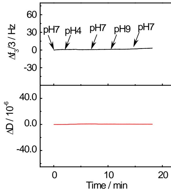
Figure S4. Frequency shift ( $\Delta f$ ) and dissipation shift ( $\Delta D$ ) of QCM-D for patterned Au nanoparticles without PDMAEMA at different pH as a function of time. This control experiment confirms that the pH response shown in Figure 3 is due to PEMAEMA brushes.
