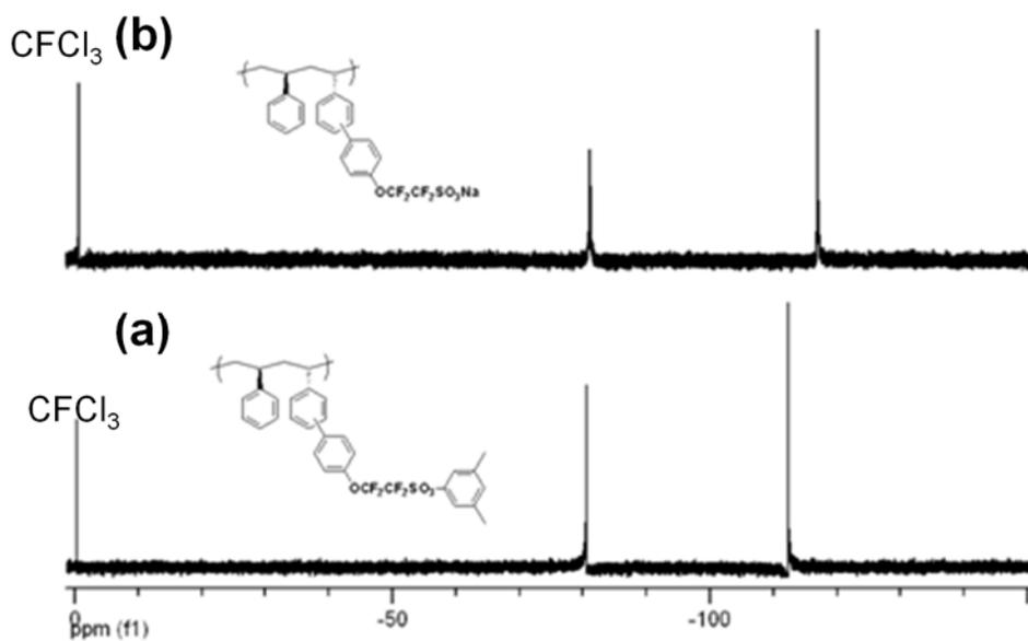
**Figure S2.**  $^{19}\text{F}$  NMR of (a) sPS-Ph (benzene- $d_6$ ) and (b) sPS-S-Na ( $\text{Na}^+$  form) (DMSO- $d_6$ ).
