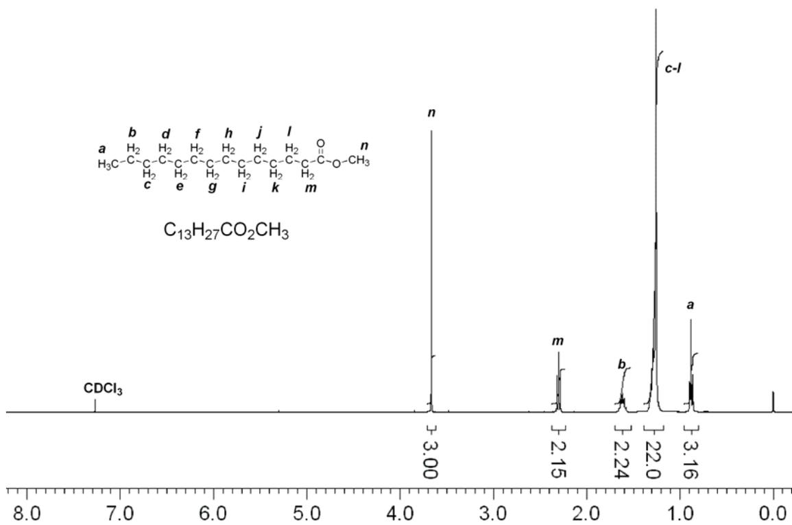
Figure S9.  $^1H$  NMR ( $CDCl_3$ ) spectrum of  $C_{13}H_{27}CO_2CH_3$ .
