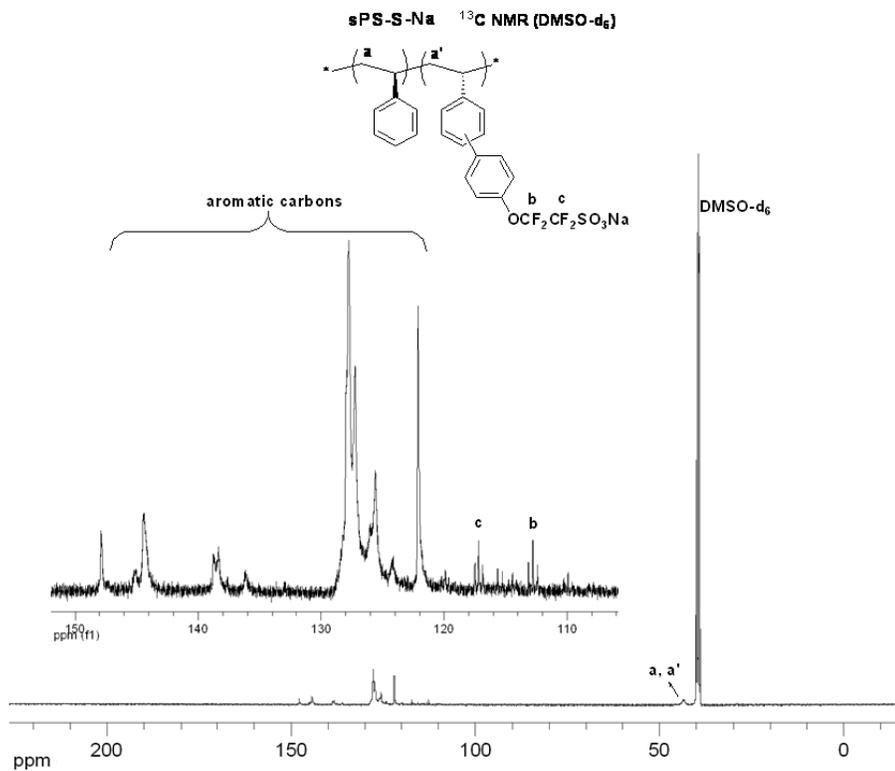
Figure S6.  $^{13}\text{C}$  NMR (DMSO- $d_6$ ) spectrum of sPS-S-Na.
