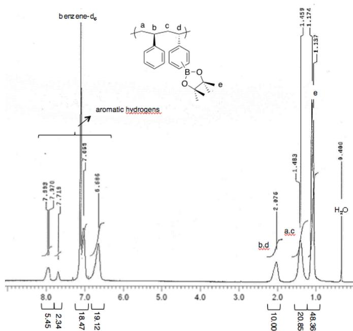
Figure S4. <sup>1</sup>H NMR (benzene-*d*<sub>6</sub>) spectrum of sPS-Bpin.
