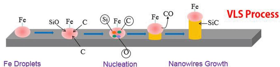
**Figure S1.** Schematic growth mechanism for the SiC nanowires under Fe-assisted condition.
