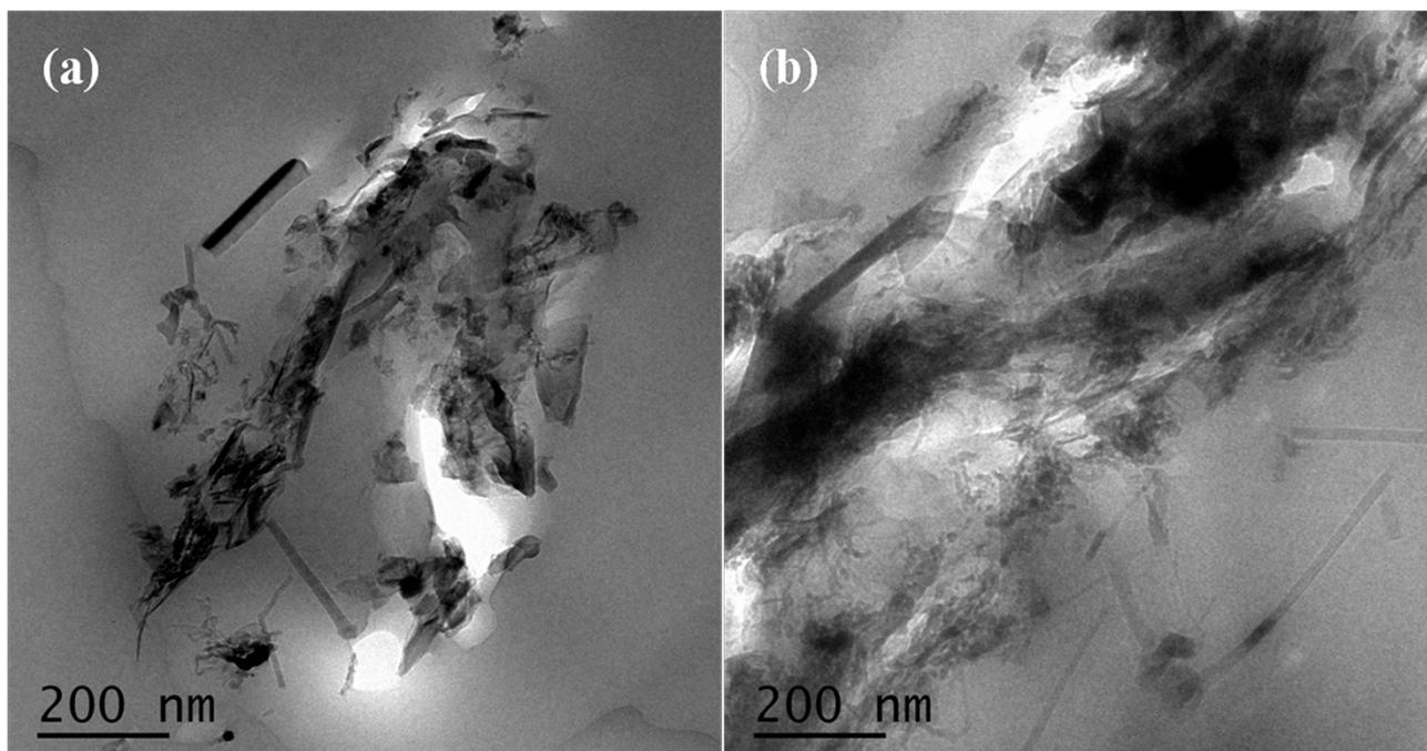
**Figure S3.** TEM images of epoxy composites with SiC<sub>NWs</sub>-GNPs nanofiller: (a) 0.5 wt%, (b) 4 wt%.
