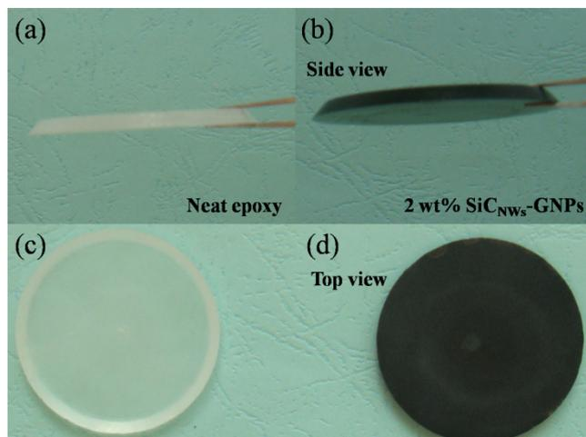
**Figure S2.** Side view of: (a) neat epoxy and (b) epoxy composite at 2 wt% SiC<sub>NWs</sub>-GNPs nanofiller loading, top view of: (c) neat epoxy and (d) epoxy composite at 2 wt% nanofiller loading.
