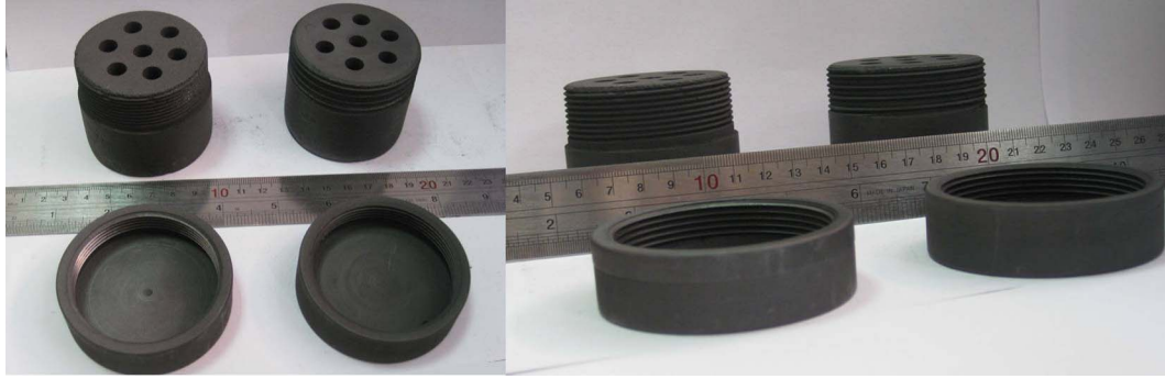
Fig. S1 A picture of the B 4 C/graphite crucible (BGC)
