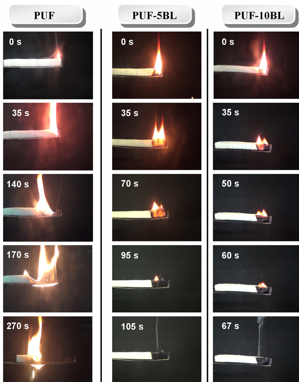
Figure S1. Snapshots showing horizontal burning tests of PUF, PUF-5BL and PUF-10BL
