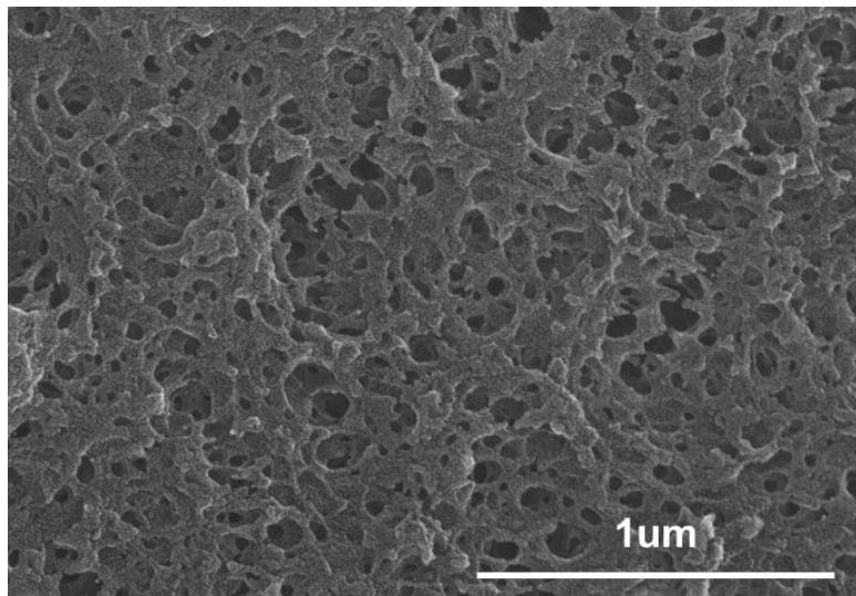
**Fig. S7.** A FE-SEM photograph verifying long-term, structural stability of SF-NW separator ( $\text{SiO}_2/\text{PVdF-HFP} = 90/10$  w/w) after 100<sup>th</sup> cycle.
