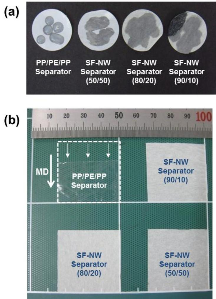
**Fig. S3.** (a) Photographs showing liquid electrolyte (1 M LiPF<sub>6</sub> in EC/DEC = 1/1 v/v) wetting behavior; (b) Thermal shrinkage of various SF-NW separators and PP/PE/PP separator after exposure to 150 °C for 0.5 h.
