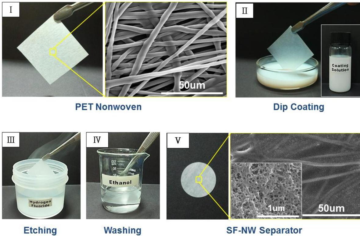
**Fig. S1.** An overview of stepwise fabrication procedure of SF-NW separators, wherein a FE-SEM photograph of a pristine PET nonwoven is provided.
