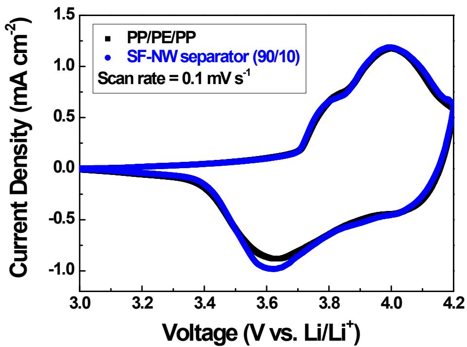
**Fig. S5.** Cyclic voltammograms of SF-NW separator ( $\text{SiO}_2/\text{PVdF-HFP} = 90/10$  w/w) and PP/PE/PP separator at a voltage scan rate of  $0.1 \text{ mV s}^{-1}$ .
