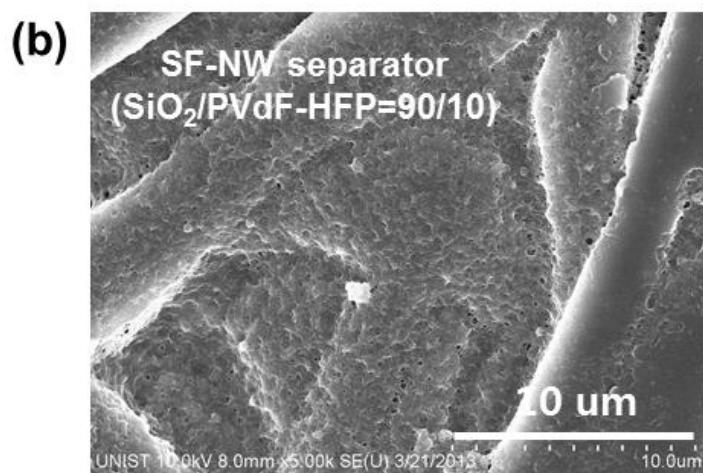
**Fig. S6.** Surface morphology of separators (after going through the test of charge rate capability): (a) PP/PE/PP separator; (b) SF-NW separator.
