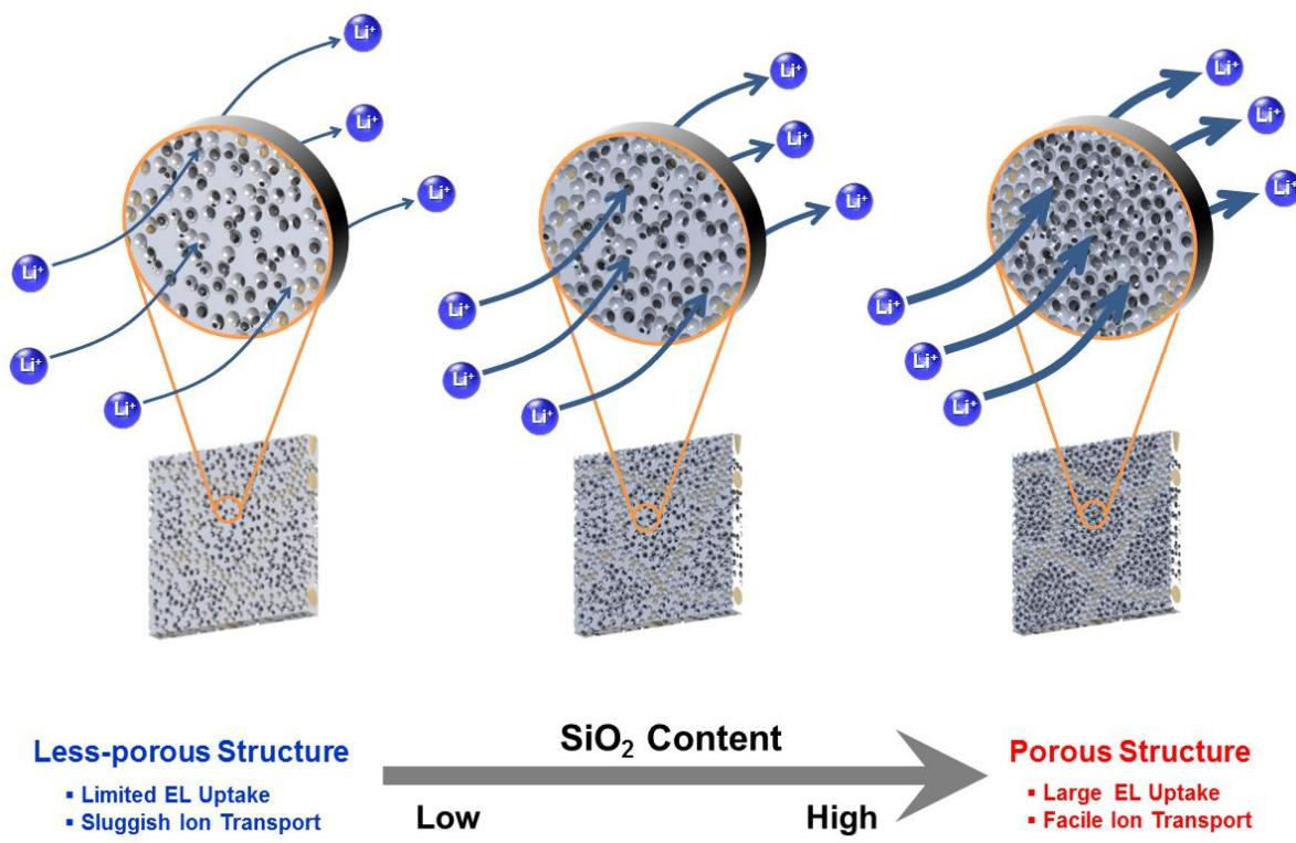
**Fig. S2.** A schematic illustration describing  $\text{SiO}_2/\text{PVdF-HFP}$  composition ratio-dependent structural variation of SF-NW separators and its influence on ionic transport.
