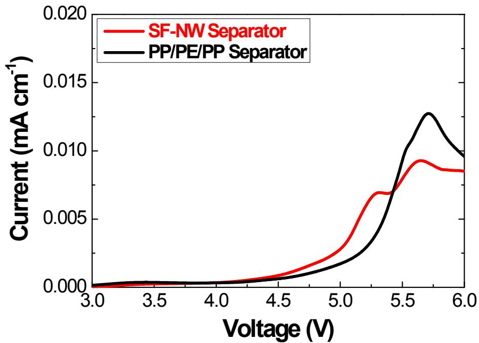
**Fig. S4.** Linear sweep voltammograms of SF-NW separator ( $\text{SiO}_2/\text{PVdF-HFP} = 90/10 \text{ w/w}$ ) and PP/PE/PP separator at a voltage scan rate of  $1.0 \text{ mV s}^{-1}$ .
