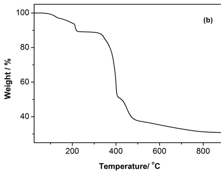
**Figure S3.** TGA curves of **1(a)** and **3(b)**.
