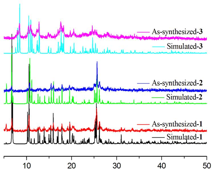
**Figure S4.** XRPD patterns of simulated and as-synthesized of **1-3**.
