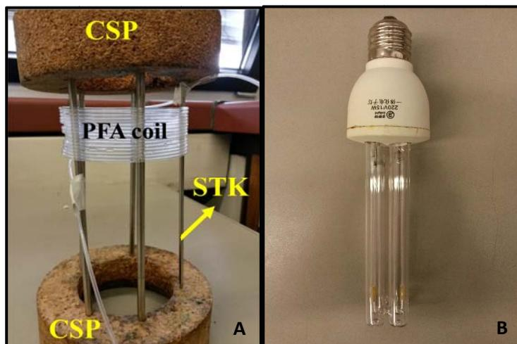
**Figure S1:** A- Support for the photoreactor. Two round bottom flask cork supports (CSP) with 5.5 cm of diameter were connected using five metal sticks (STK). The PFA tube was coiled around the support; B- commercial germicide compact fluorescent UV light.
