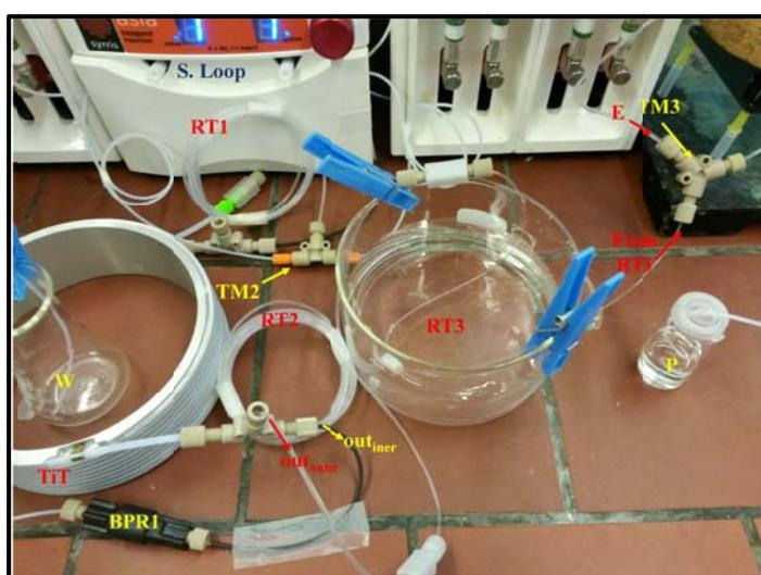
**Figure S4:** Detail of the setup. RT1 (1 mL coil reactor); TiT (tube-in tube reactor); TM2 (T-mixer 2); RT2 (4mL coil reactor), RT3 (2 mL coil of gas-permeable Teflon AF-2400 in a bath of AcOH in MeOH); TM3 (T-mixer 3); E (feed of nucleophile); W (quench solution of AcOH); BPR1 (back-pressure regulator 1); P (collected product)
