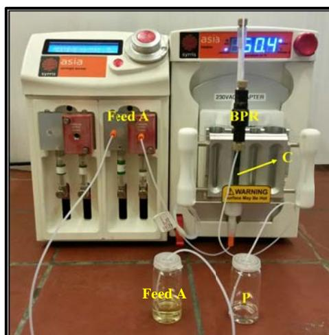
**Figure S5:** Feed A (0.1 M solution of diazoketone **3** in THF/EtOH 1:1) was pumped through the column (**C**), at 60 °C. Collected product (**P**).
