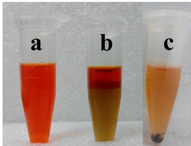
**Fig. S1** The photo of AST in acetic ether (a), stratification of the mixing solution of AST in acetic ether (upper layer) and GO in water (lower layer) (b), and extraction of AST from freeze-dried GO-AST by dichloromethane (c).
