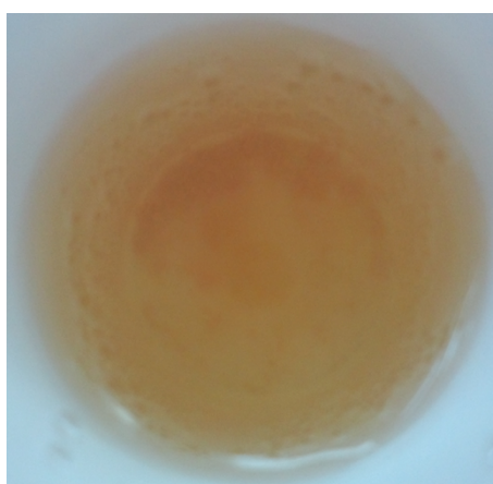
Fig. S2 The products of WPBs which were hydrothermally treated in 5.0 wt% H 2 O 2 solution at 180 °C for 12 h. Note that many bubbles generated and adhered to the wall of the autoclave.
