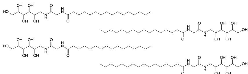
**Fig. S6** Schematic illustration of interdigitated lamellar packing in **SG-G**.
