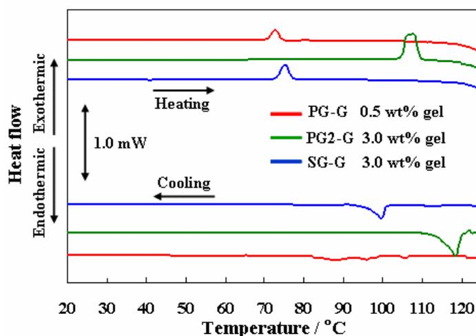
**Fig. S2** DSC curves of hydrogels (2 °C/min).
