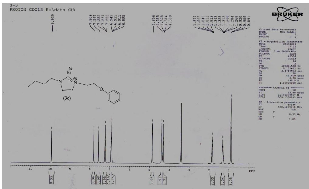
Figure 1.7: 1 H NMR spectra of 1-butyl-3-(2-phenoxyethyl)-1 H -imidazol-3-ium bromide (3c)
