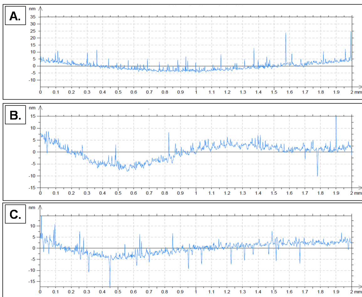
Figure S1. Mean surface profile recorded at 50\text{ }\mu\text{m/s} scan rate over 2\text{ mm} \times 2\text{ mm} surface of pristine (A), acidic treated (B) and, acidic and thermal treated (C) DMSO doped SF film. Each mean profile is averaged over 10 scans.
