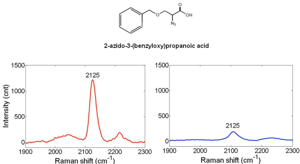
**Figure S1:** Raman scattering of the azido group from 2-azido-3-(benzyloxy)propanoic acid. (left) Typical experimental SERS of  $1 \mu\text{M}$  ( $3 \text{ pmol}$ ) solution deposited on Klarite substrate and (right) the corresponding reference Raman spectrum of 100 mM ( $300 \text{ pmol}$ ) solution deposited on an aluminum coated slide.
