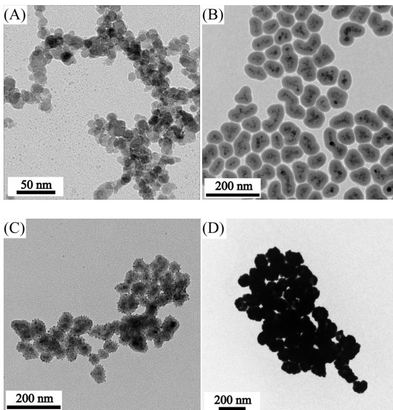
Fig. S4 TEM images of (A)  $\text{Fe}_3\text{O}_4$  nanoparticles, (B)  $\text{Fe}_3\text{O}_4@SiO_2$  core-shell nanoparticles, (C)  $\text{Fe}_3\text{O}_4@SiO_2@Au$  seeds, (D)  $\text{Fe}_3\text{O}_4@SiO_2@Au$  shell nanoparticles (GMNPs).
