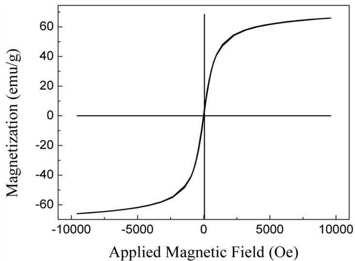
Fig. S3 Magnetic hysteresis curve of  $\text{Fe}_3\text{O}_4$  nanoparticles.
