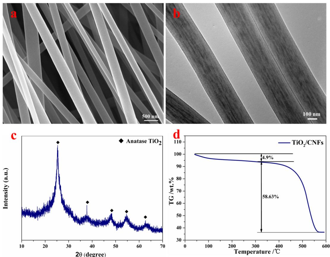
Fig.S1 (a) SEM and (b) TEM images, (c) XRD patterns and (d) TGA curves of anantase  $\text{TiO}_2/\text{CNFs}$ .
